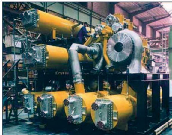
Figure 4-10: 8 Stage Integrally Geared Compressor (Courtesy of MAN Turbo 7 )
