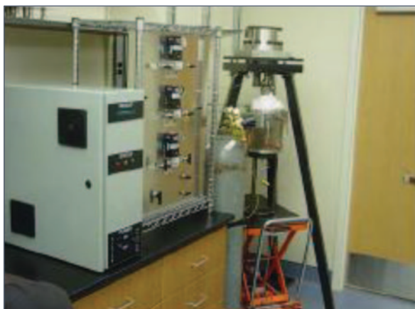
Figure 1: Modified TGA for CO 2 Sorbent Testing
