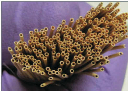
Figure 2: Image of a Bundle of PBI-Based, Asymmetric Hollow Fibers
