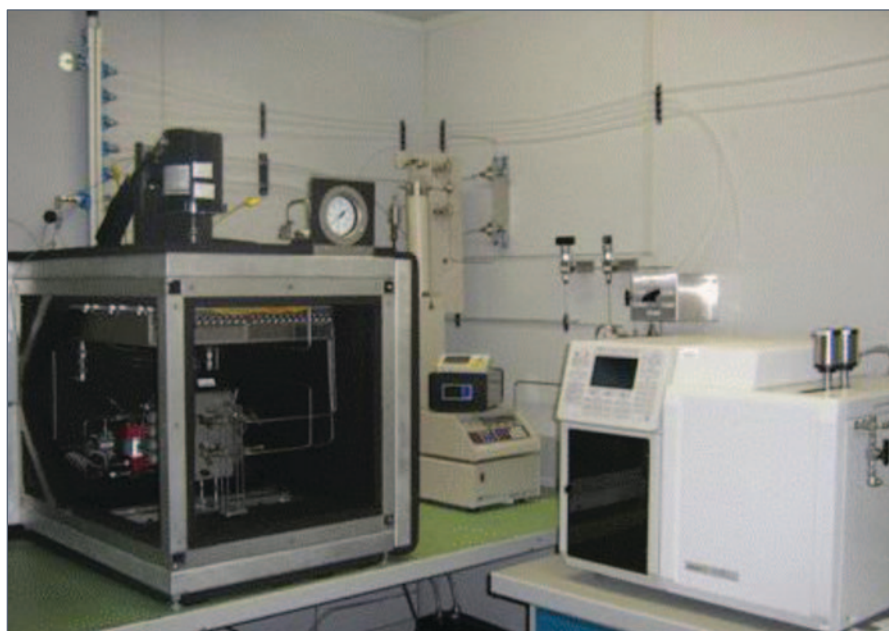
Figure 3: CanmetENERGY's High-Pressure CO 2 Test Cell and Bench-Scale Facility
