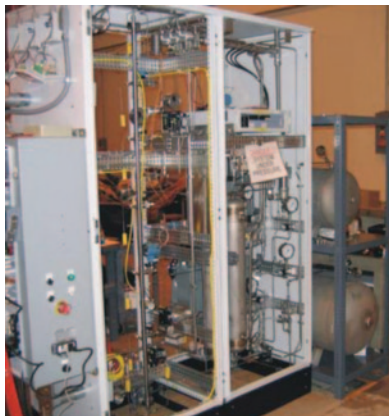
Figure 1: Fixed-Bed Reactor Skid
