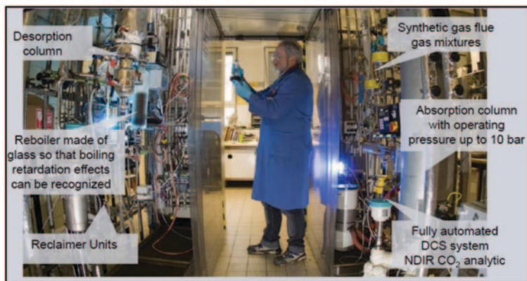
Figure 1: Siemens Lab Plant for CO 2 Capture Tests at Frankfurt Hoechst Industrial Park
