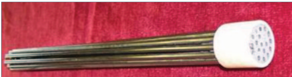
Figure 2: Candle Filter Configuration for CMS Membrane and Module (pilot scale)
