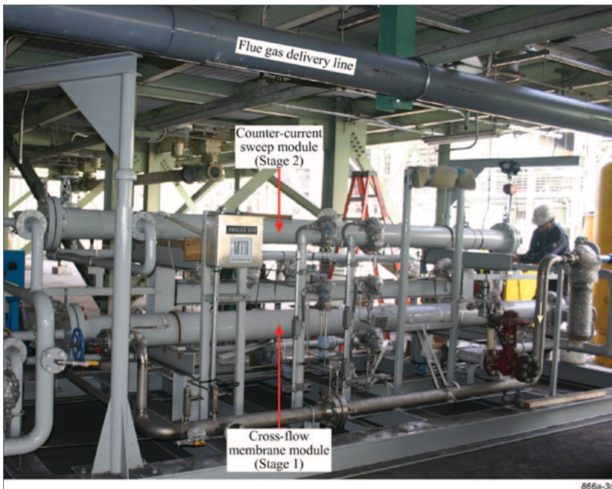
Figure 4: Membrane Skid Used for Pilot-Scale Slipstream Testing at the APS Cholla Power Plant
