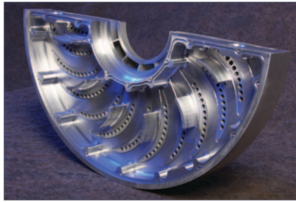
Figure 6: Internally Cooled Compressor Diaphragm
