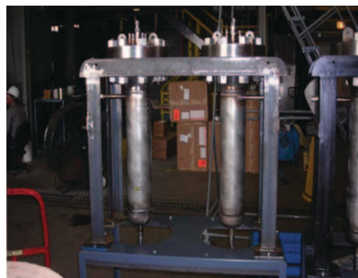
Figure 1: Heated Fixed-Bed Reactors
