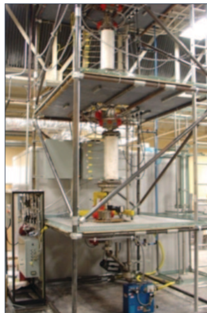
Figure 2: Sub-Pilot Scale (25 kWth) CDCL Unit
