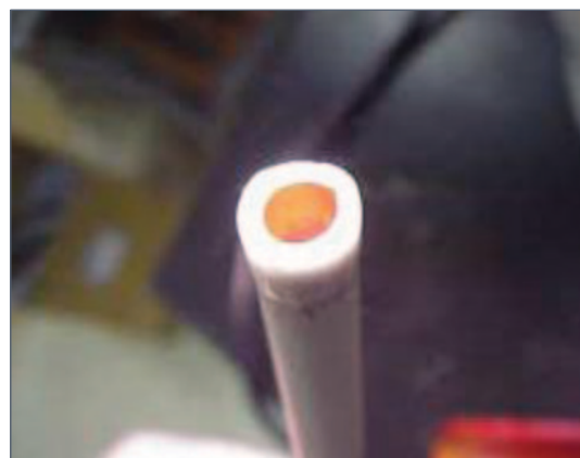
Figure 1: Unheated, Broken Pd-Cu/-Alumina Composite Membrane
