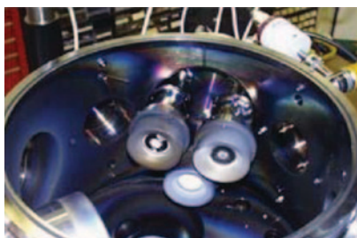
Figure 1: A Co-Sputtering Chamber
