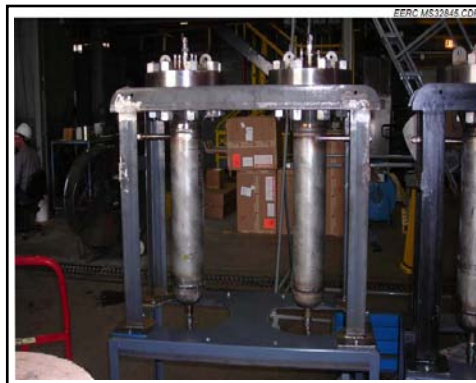
Figure 1: Heated Fixed-Bed Reactors
