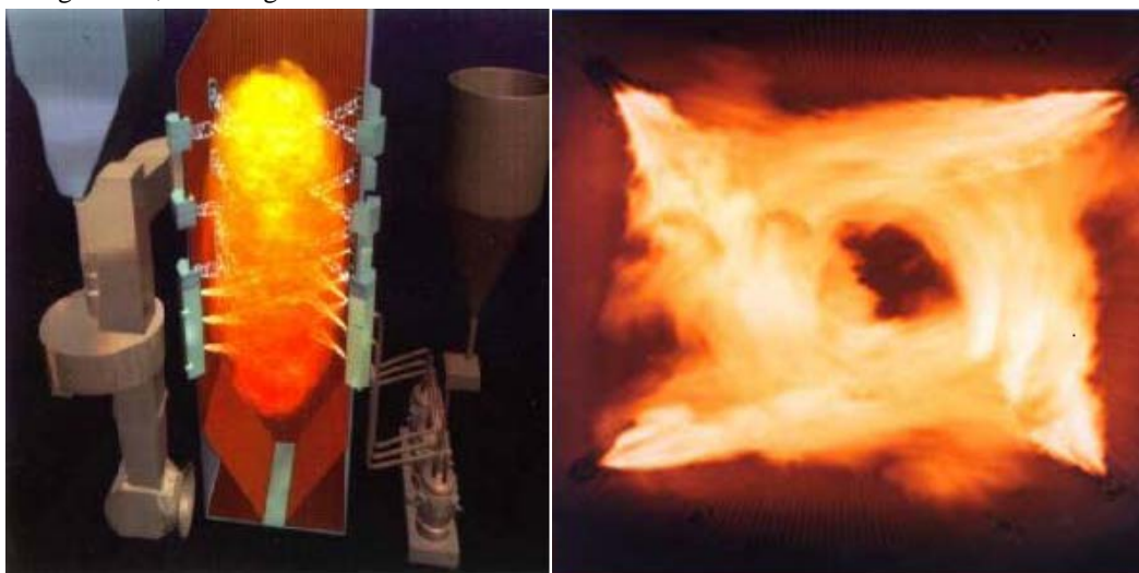
Figure 3: Model of Tangential Firing System Furnace Cavity (left); Top View of Tangential Firing (right)
