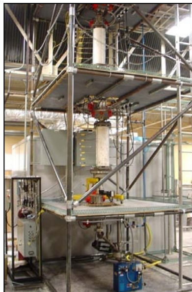
Figure 2: Sub-Pilot Scale (25-kWth) CDCL Unit
