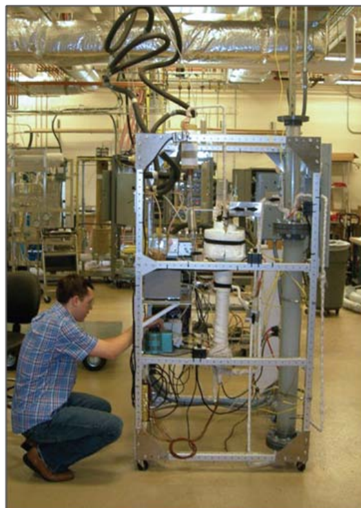
Figure 2: Lab-Scale CO 2 Absorption Reactor Skid
