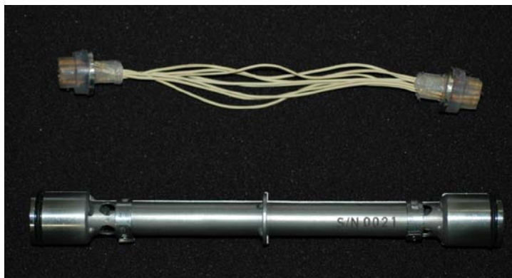
Figure 2: Image of a Bundle of PBI-Based, Asymmetric Hollow Fibers and Fiber Potting
