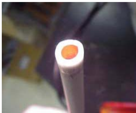
Figure 1: Unheated, Broken Pd-Cu/ \alpha -Alumina Composite Membrane
