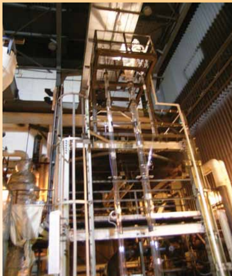
Chemical Looping Cold Flow Model
