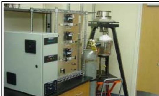
Figure 1: Modified TGA for CO 2 Sorbent Testing
