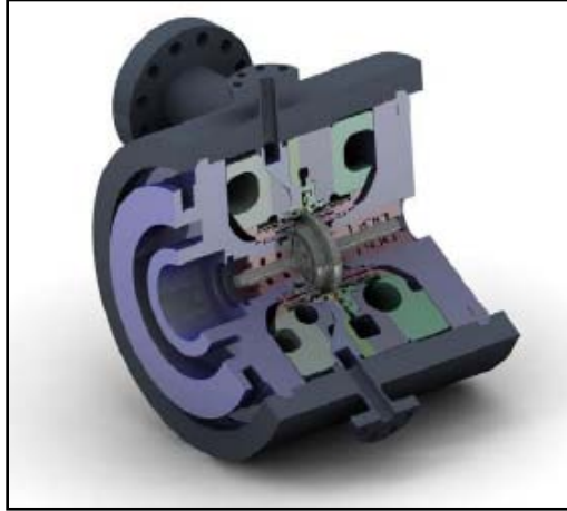
Figure 3: Cross Sectional Model of a 1/10 th Scale Single Stage Supersonic Shock Wave Compressor
