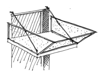
External light shelves reduce direct solar gain and reduce cooling load while improving penetration of daylighting.
