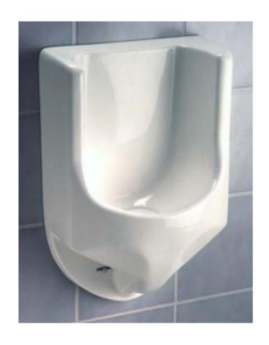
Waterless urinals are a proven technology with both first cost and long term operational cost savings. Water supply piping and flush valves are eliminated, and no water is used.
