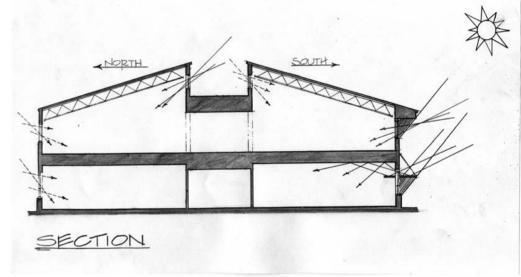
Aggressive use of day-lighting strategies and light colored paints in this building reduced the number of light fixtures and reduced cooling load resulting in both first cost savings and significant operational savings.
