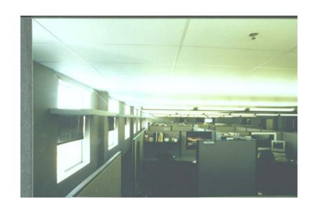
Day-lighting, light shelves, and light colored reflective ceiling reduces the number of light fixtures needed... thereby reducing lighting and electrical system costs. Less lights means less heat which reduces cooling load, equipment size and cost.
