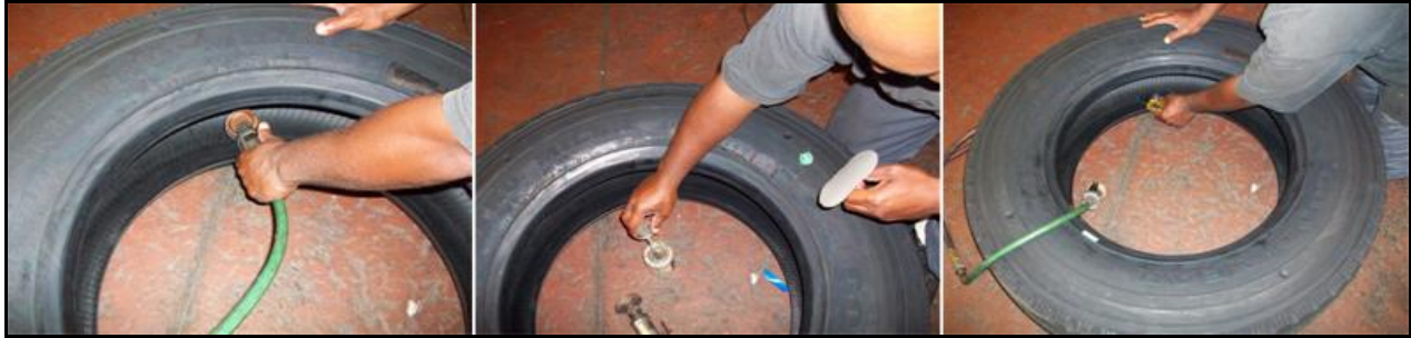
Figure 19. Michelin eTire Sensor Dock Installation Process
