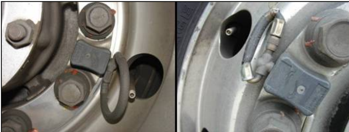
Figure 22. Improper IVTM Hose Connections
