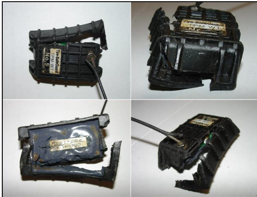
Figure 30. Additional Damaged Tire-SafeGuard Sensors
