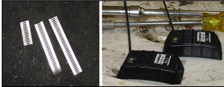
Figure 28. Tire-SafeGuard Band Fragments and Damaged Sensors, Bus Number 2508
