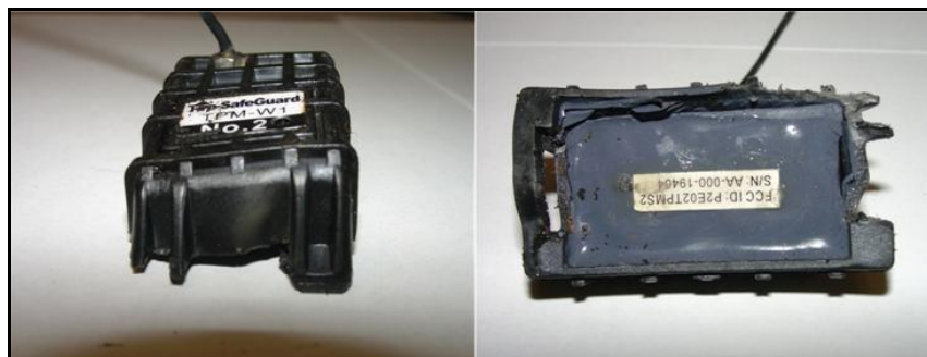
Figure 31. Additional Damaged Tire-SafeGuard Sensors
