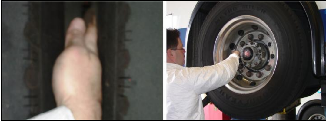
Figure 7. Wheel Gap and Cap Nut Removal on a Rear Wheel
