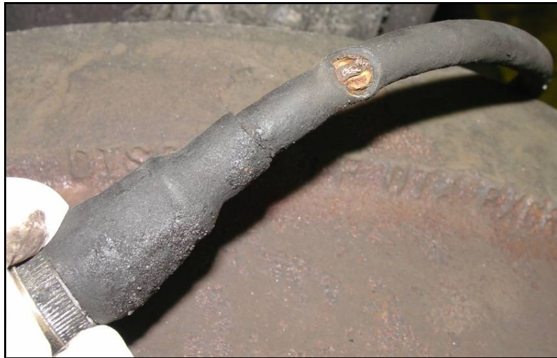
Figure 51. StrainSert Anchor Pin Cable Failure
