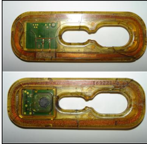
Figure 27. Cracked eTire Sensors, Bus Number 2512
