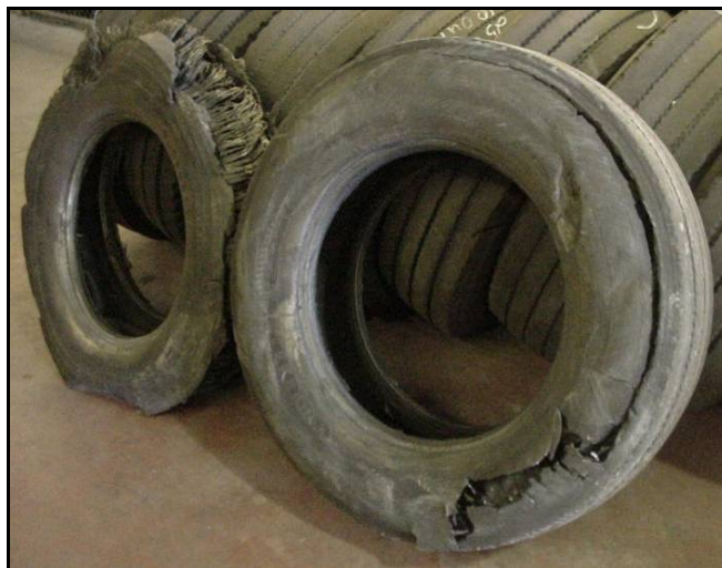
Figure 32. Damaged Tires From Bus Number 2503
