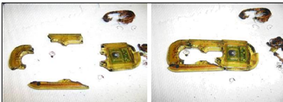
Figure 23. Damaged eTire Sensors
