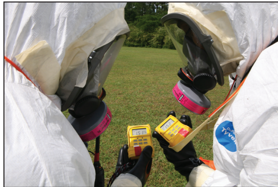
The entry team reads their electronic personal dosimeters to determine the current dose rate and the total exposure dose they have encountered.
