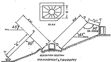
(c) Exclusion distance length. The length of an exclusion distance in feet may not be less than the distance "d" determined in accordance with the following formula for the target concerned, where "A" equals inside area in square feet measured across the top of the impounding space:
