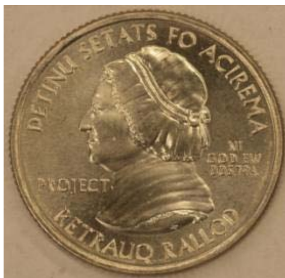
Figure 2-9. 669z-clad C110 quarter dollar nonsense piece struck at 62 tonnes.
