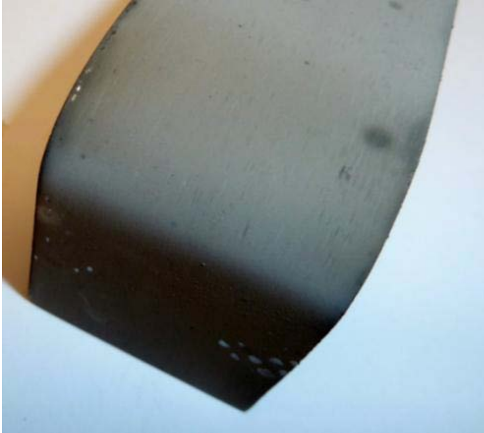
Figure 2-G-11. Carbonyl nickel-coated steel specimen after single-bend testing.
