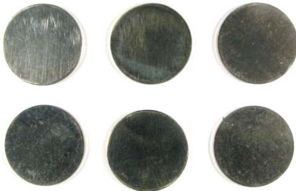
Figure 2-D-18. Steam corrosion tested incumbent dollar coin planchets.
