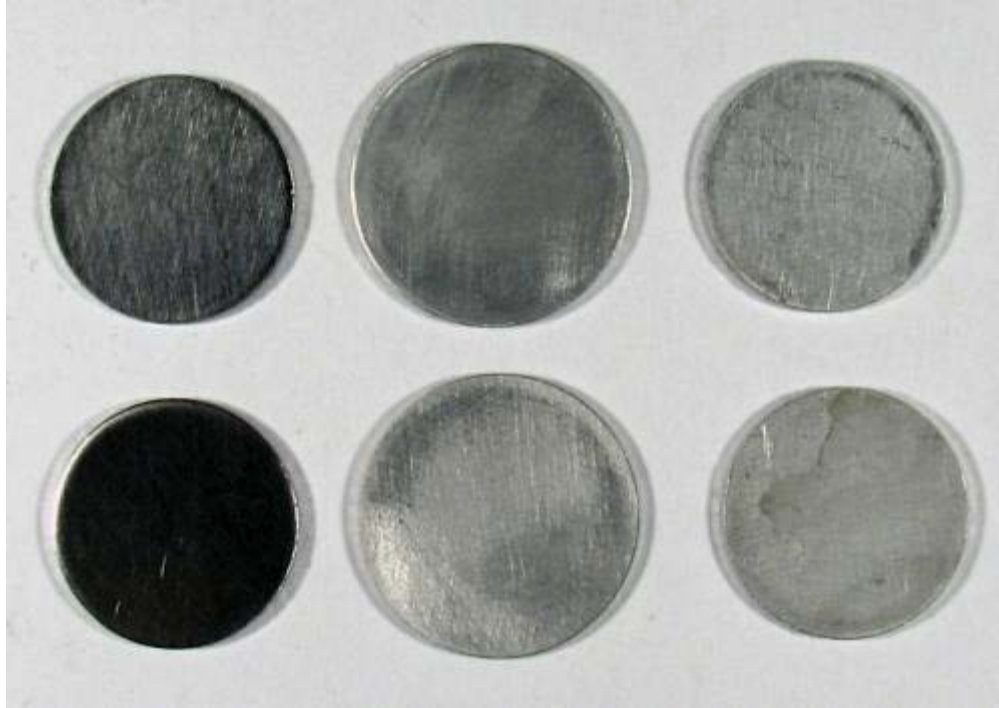
Untested, as-received on left (one-cent coin size blank), lightly sanded and tested in middle (5-cent coin size blank), and tested one-cent coin size blanks on right.
