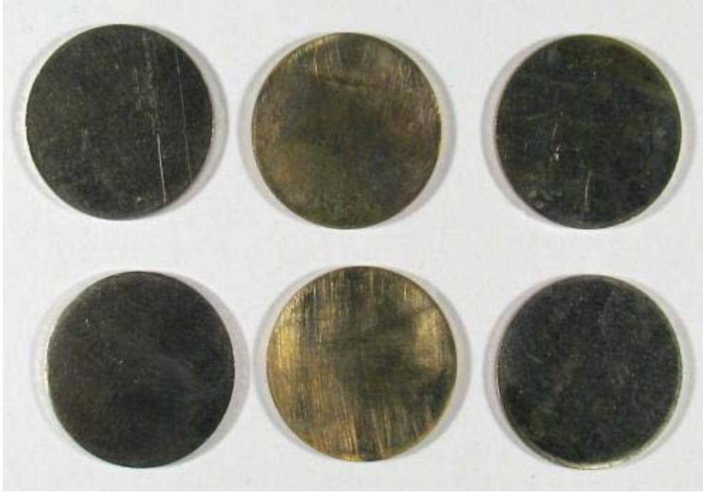
Figure 2-D-10.Steam corrosion tested G6 mod 5-cent blanks.
