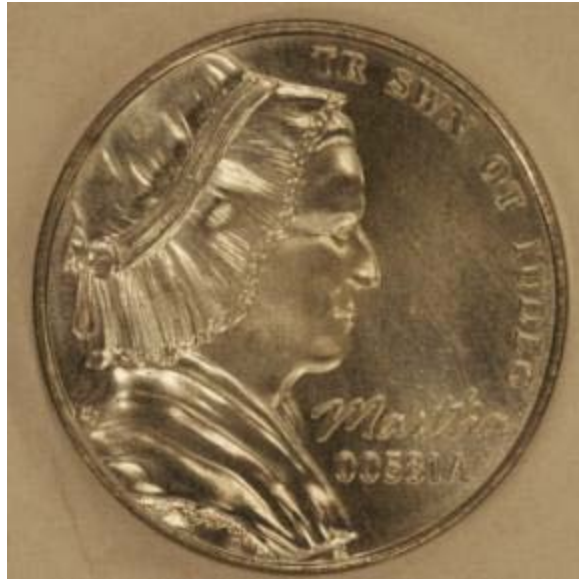
Figure 2-4. Dura-White-plated zinc 5-cent nonsense piece struck at 54 tonnes.
