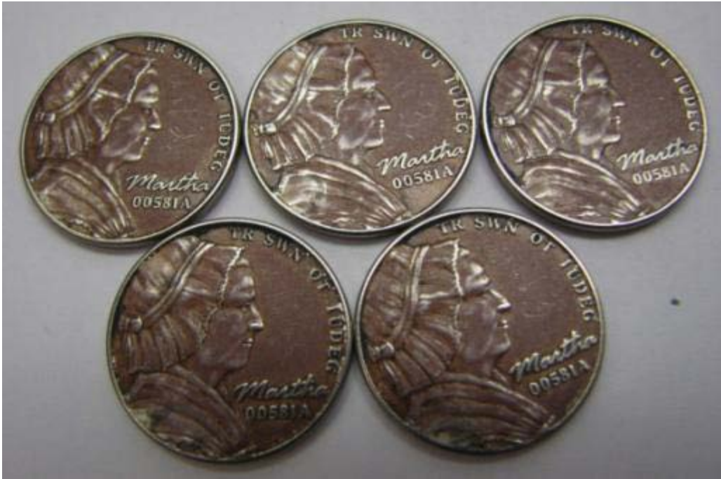
Figure 2-F-8. Wear tested 5-cent nonsense pieces (incumbent material).
