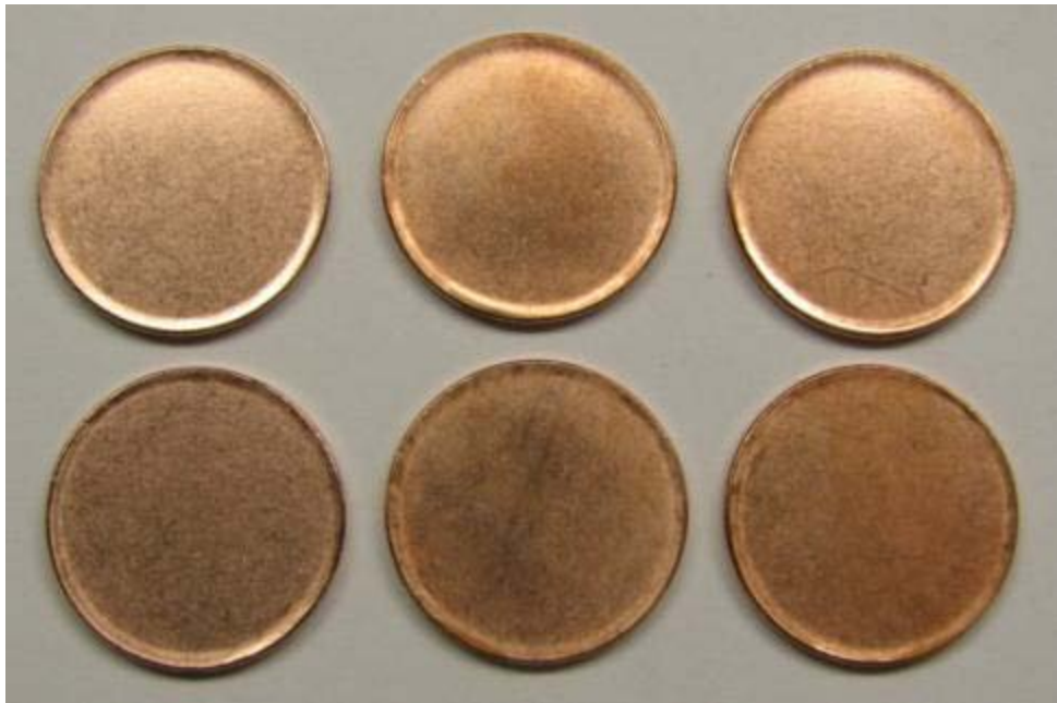
Figure 2-D-2. Steam corrosion tested copper-plated steel one-cent planchets from Jarden Zinc Products.
