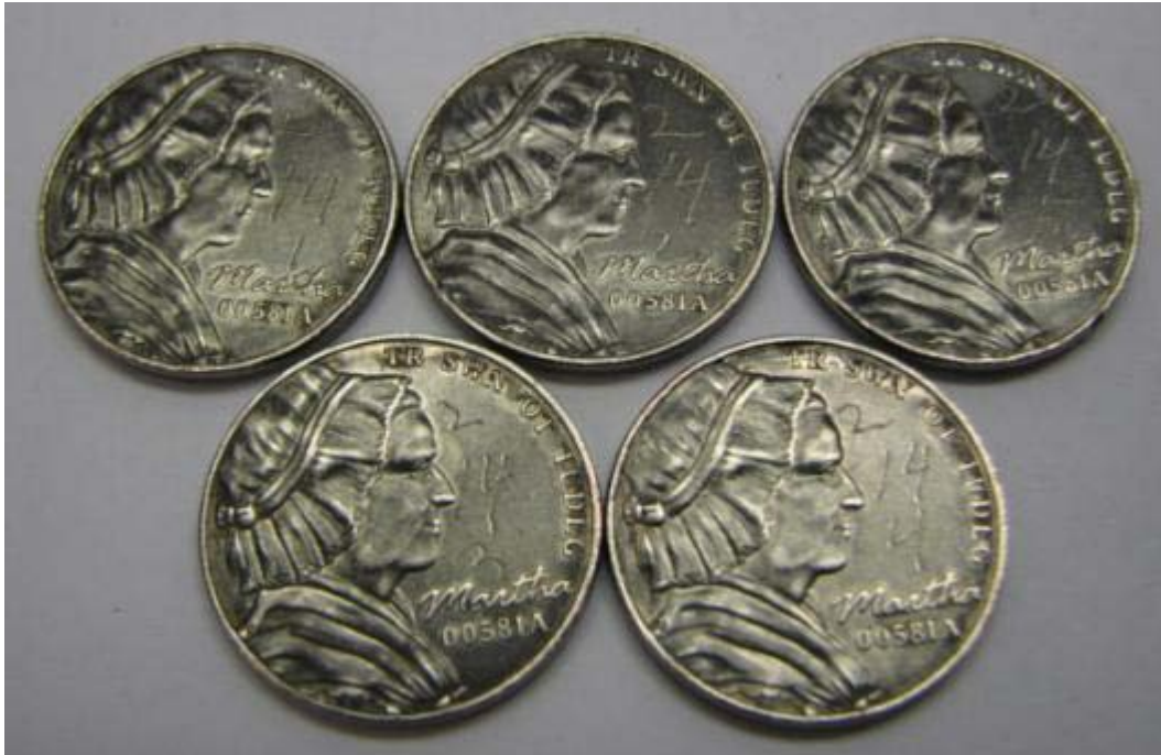
Figure 2-F-10. Wear tested Multi-Ply-plated steel 5-cent nonsense pieces.
