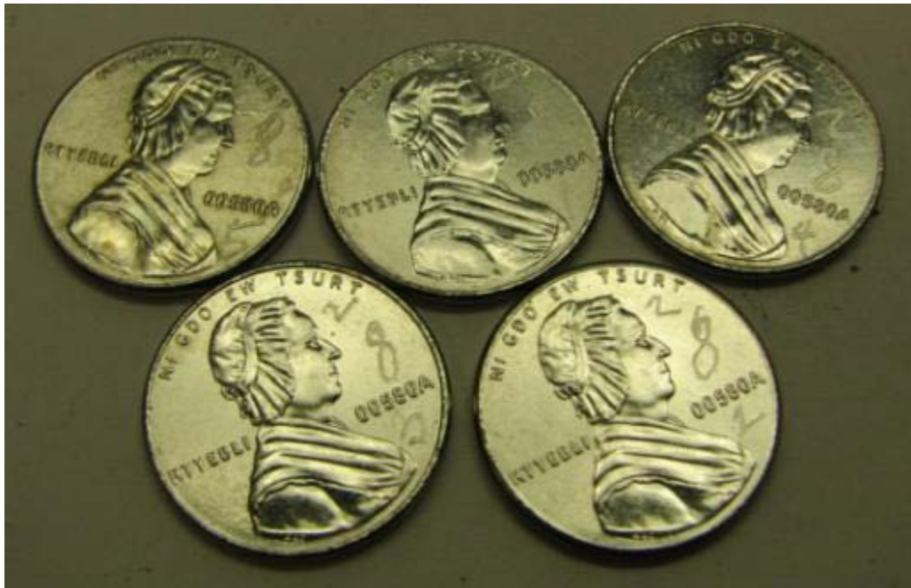
Figure 2-F-6. Wear tested aluminized steel (Ryerson) one-cent nonsense pieces.
