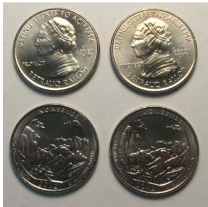
Two pieces on left are as-struck and two on right are after a 2-hour steam corrosion test. Figure 2-E-19. Steam corrosion tested Multi-Ply-plated steel quarter dollar nonsense pieces.
