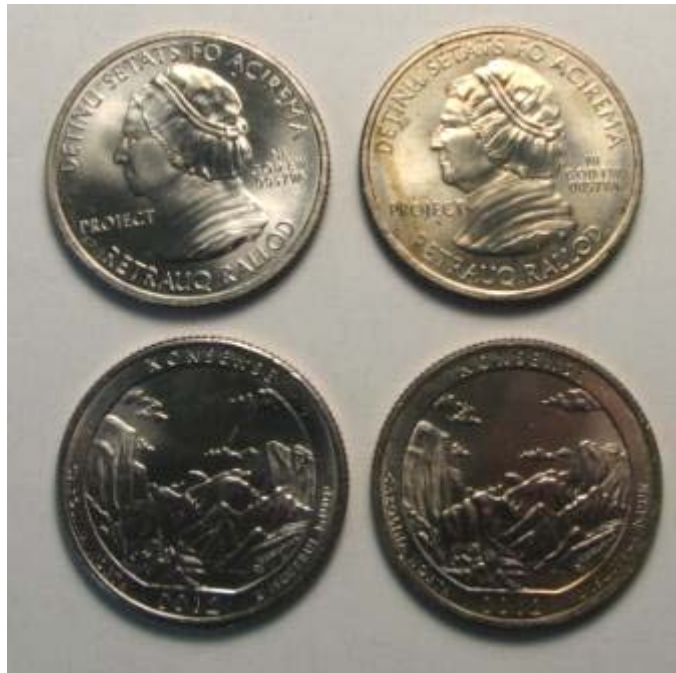
Two pieces on left are as-struck and two on right are after a 2-hour steam corrosion test. Figure 2-E-18. Steam corrosion tested quarter dollar nonsense pieces (incumbent material).
