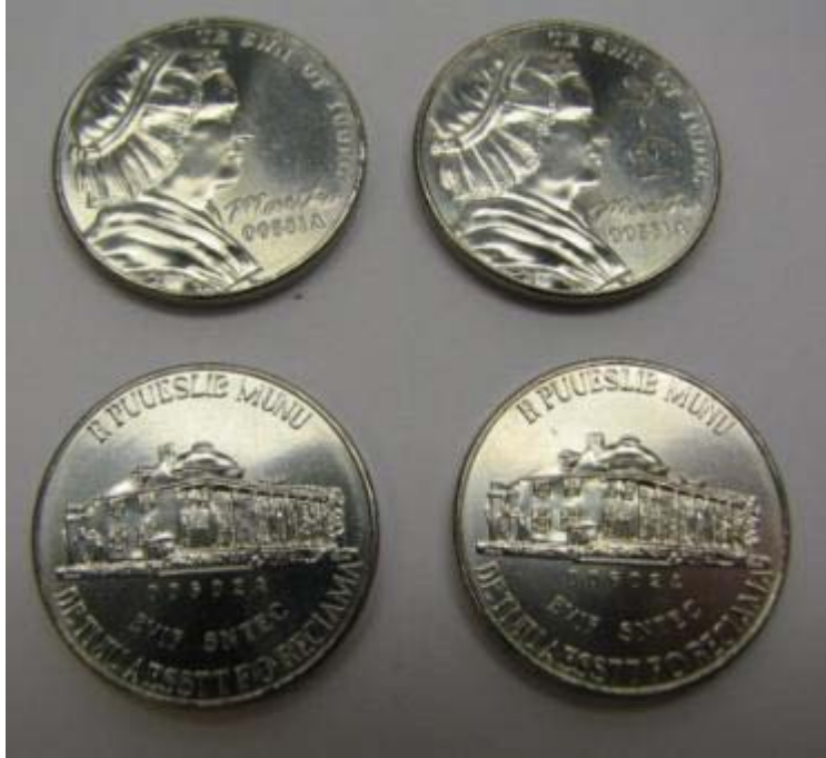
Two pieces on left are as-struck and two on right are after a 2-hour steam corrosion test. Figure 2-E-16. Steam corrosion tested nickel-plated 31157 5-cent nonsense pieces.
