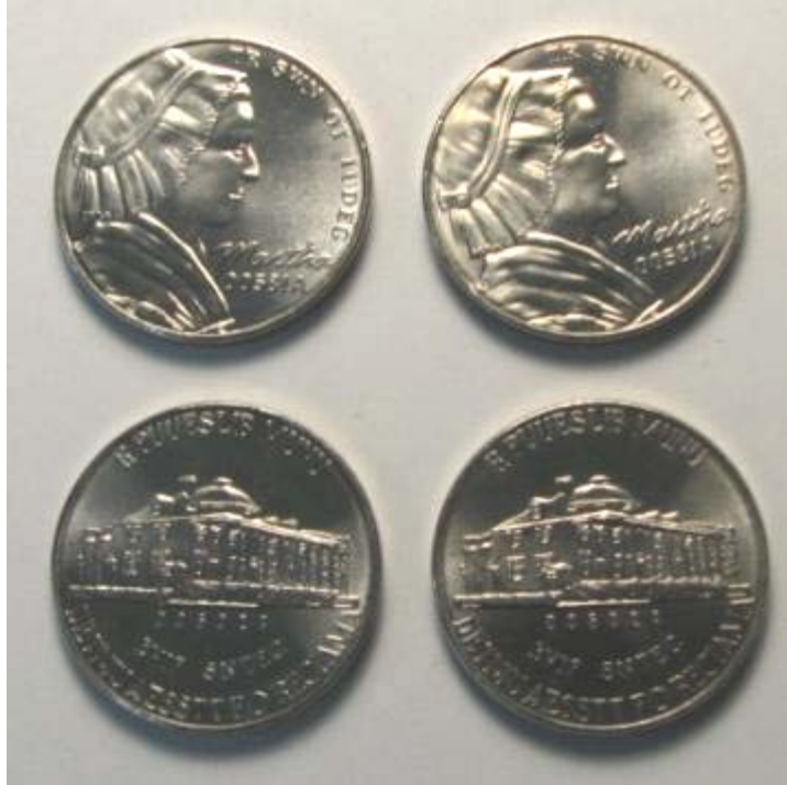
Two pieces on left are as-struck and two on right are after a 2-hour steam corrosion test. Figure 2-E-10. Steam corrosion tested Multi-Ply-plated steel 5-cent nonsense pieces.
