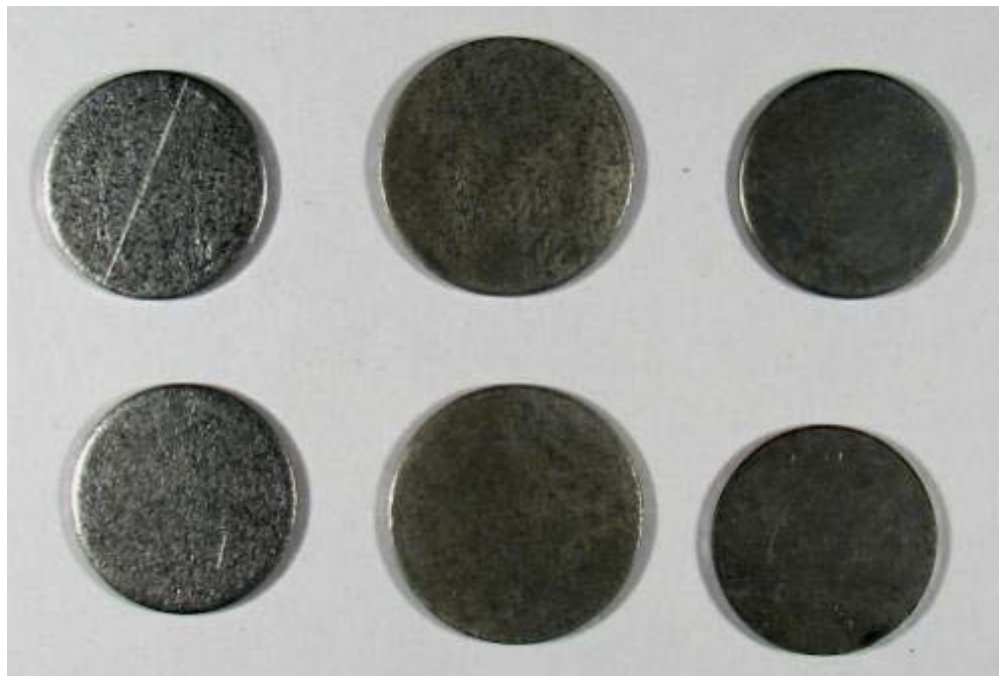
Untested, as-received on left (one-cent coin size blank), lightly sanded and tested in middle (5-cent coin size blank), and tested one-cent coin size blanks on right.
