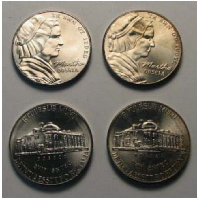
Figure 2-E-8. Steam corrosion tested 5-cent nonsense pieces (incumbent material).
