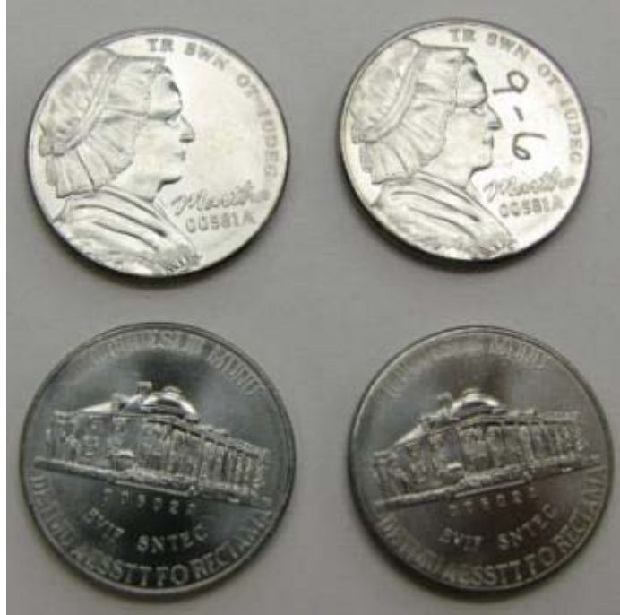
Figure 2-E-14. Steam corrosion tested 430 stainless steel 5-cent nonsense pieces.
