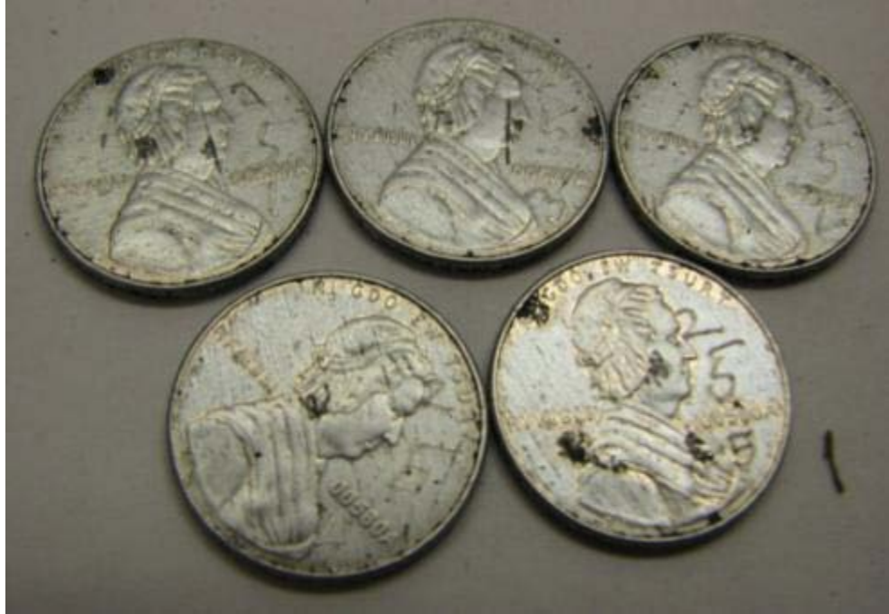
Figure 2-F-4. Wear tested 5052-H32 one-cent nonsense pieces.
