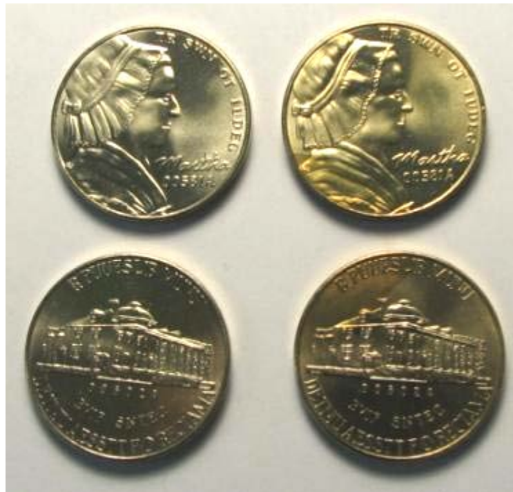
Two pieces on left are as-struck and two on right are after a 2-hour steam corrosion test. Figure 2-E-17. Steam corrosion tested unplated 31157 5-cent nonsense pieces.
