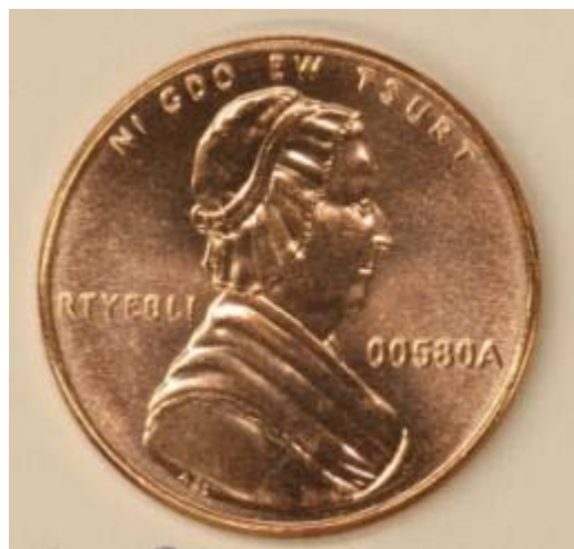
Figure 2-14. Copper-plated steel one-cent nonsense piece struck at 40 tonnes from planchets supplied by JZP.
