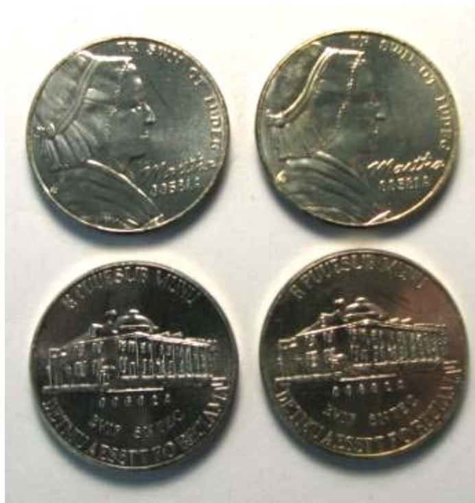
Figure 2-E-12. Steam corrosion tested G6 mod 5-cent nonsense pieces.
