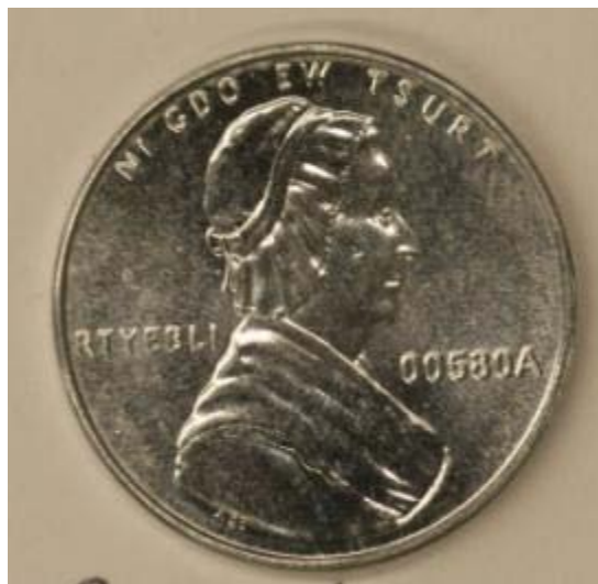
Figure 2-G-1. A26-coated A190 one-cent nonsense piece struck at 40 tonnes.
