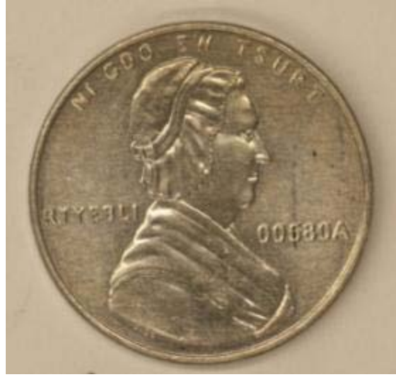
Figure 2-12. 5052-H32 one-cent nonsense piece struck at 25 tonnes.
