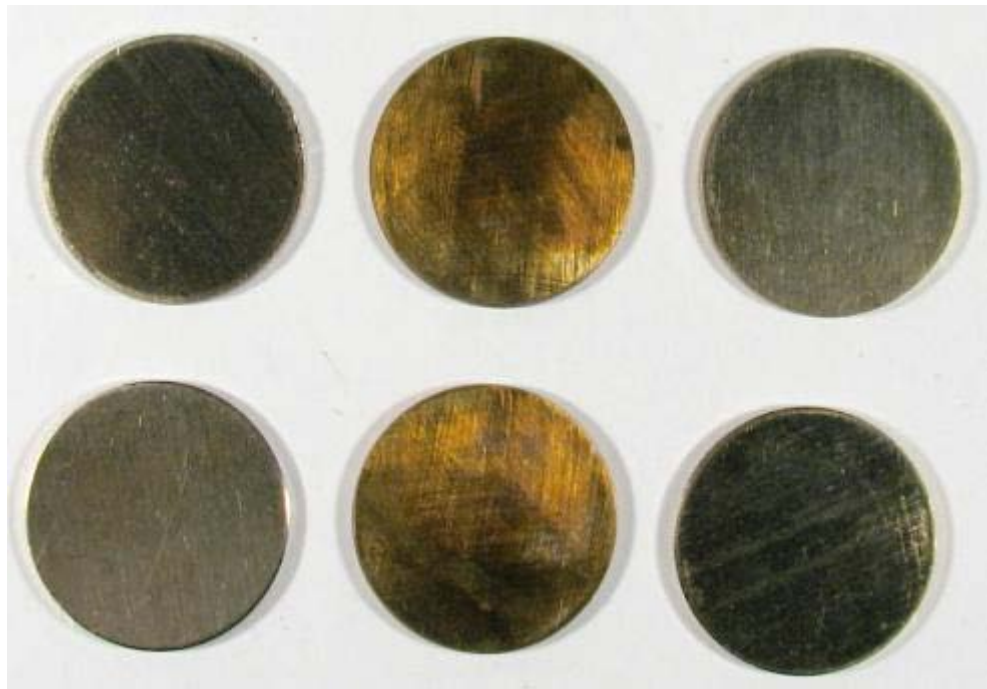
Figure 2-D-10.Steam corrosion tested G6 mod 5-cent blanks.
