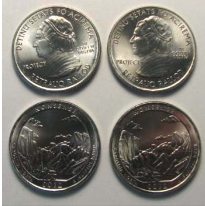
Two pieces on left are as-struck and two on right are after a 2-hour steam corrosion test. Figure 2-E-20. Steam corrosion tested nickel-plated steel quarter dollar nonsense pieces.
