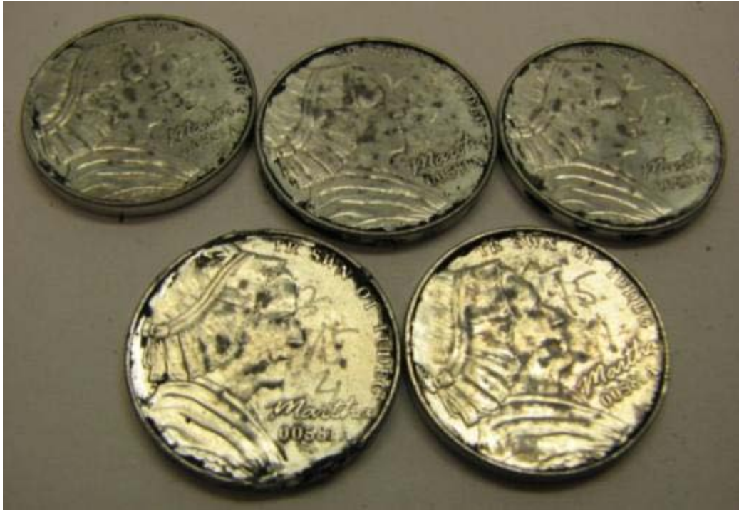
Figure 2-F-8. Wear tested 5-cent nonsense pieces (incumbent material).
