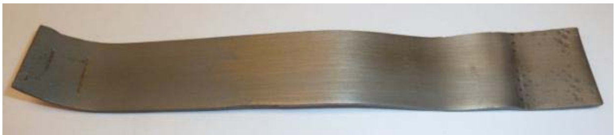
Figure 2-G-14. Carbonyl nickel deposited on C110 strip bent back and forth several times.
