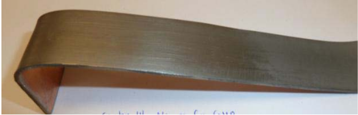
Figure 2-G-13. Single bend test of carbonyl nickel deposited on C110.
