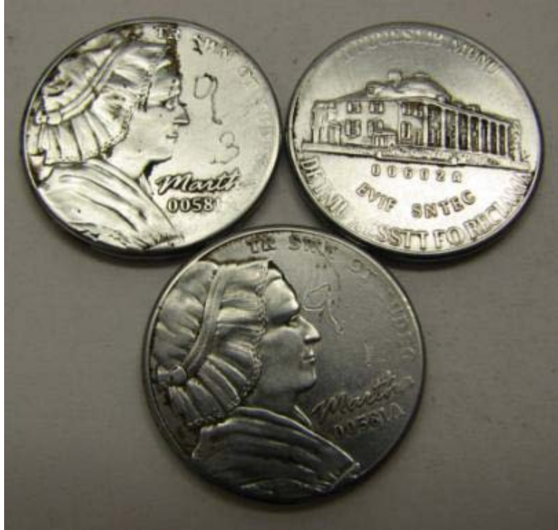
Minor wear (note that design was not filled during striking trial in spite of excessive coining load).
