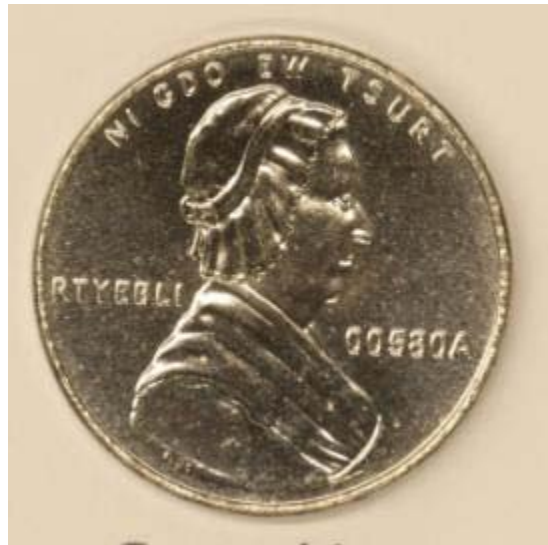
Figure 2-11. 302HQ stainless steel one-cent nonsense piece struck at 60 tonnes.
