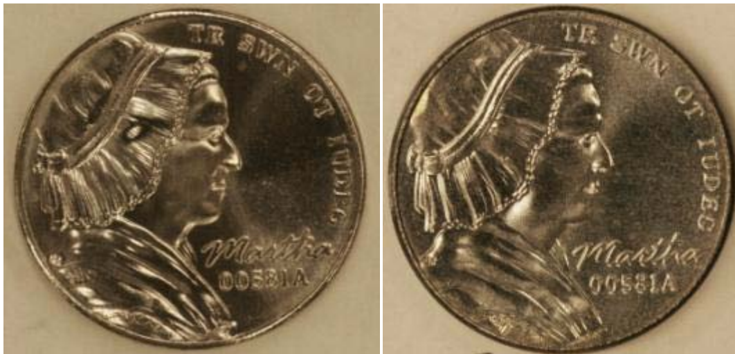
(a) Standard anneal – blanked at CTC (b) Alternative anneal – blanked at Carpenter Technology
