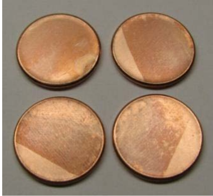
Figure 2-G-7. Type II A26-coated copper-plated zinc one-cent planchets before (left) and after (right) steam corrosion testing.
