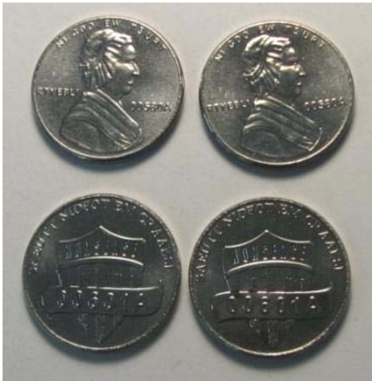
Two pieces on left are as-struck and two on right are after a 2-hour steam corrosion test. Figure 2-E-7. Steam corrosion tested 302HQ stainless steel one-cent nonsense pieces.
