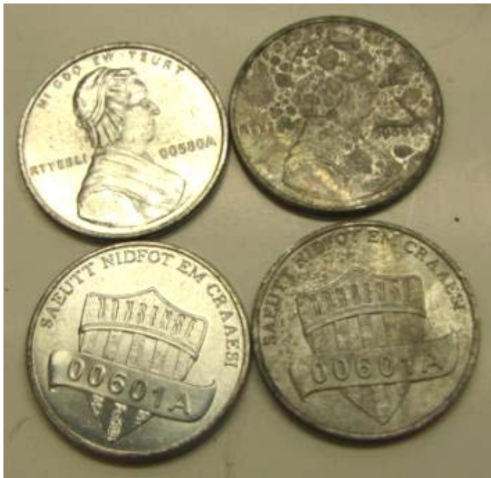
Figure 2-E-4. Steam corrosion tested 5052-H32 one-cent nonsense pieces.
