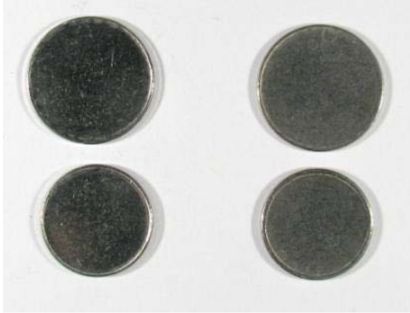
As-received on left and ready-to-strike and tested on right, quarter dollar plachet on top and 5-cent plachet on bottom.
