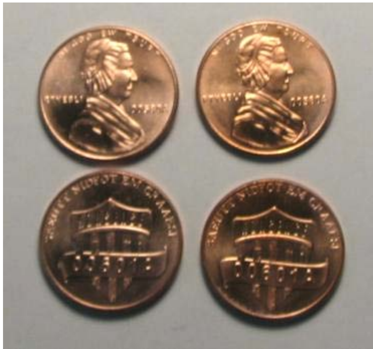
Figure 2-E-1. Steam corrosion tested one-cent nonsense pieces (incumbent material).
