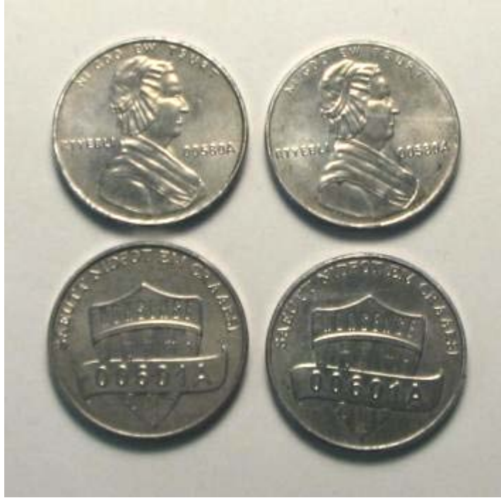
Figure 2-E-4. Steam corrosion tested 5052-H32 one-cent nonsense pieces.
