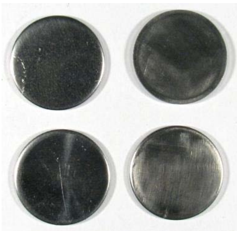
Figure 2-D-12.Steam corrosion tested 430 stainless steel 5-cent blanks.
