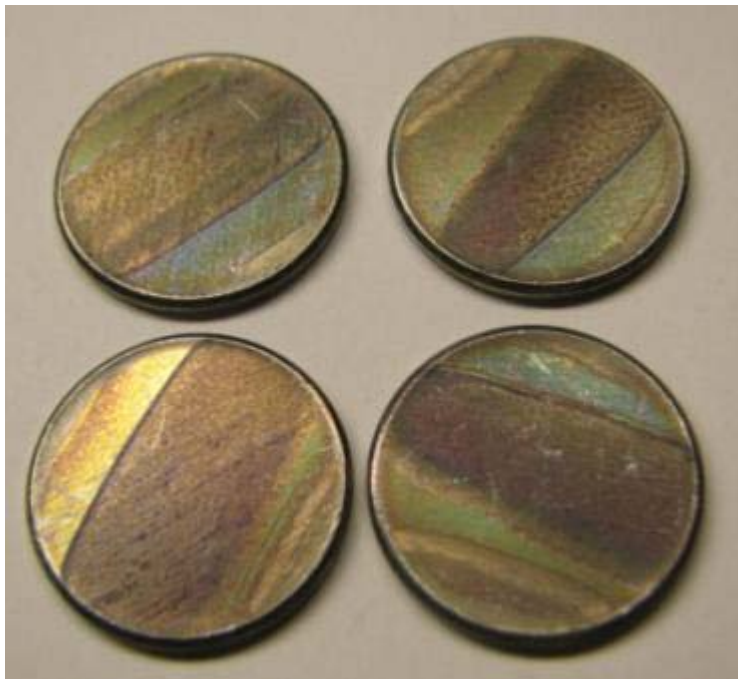
Figure 2-G-6. Type II A26-coated A190 one-cent planchets before (left) and after (right) steam corrosion testing.
