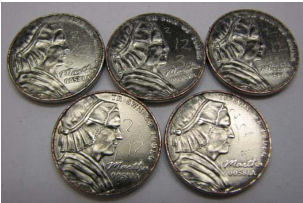
Figure 2-F-10. Wear tested Multi-Ply-plated steel 5-cent nonsense pieces.
