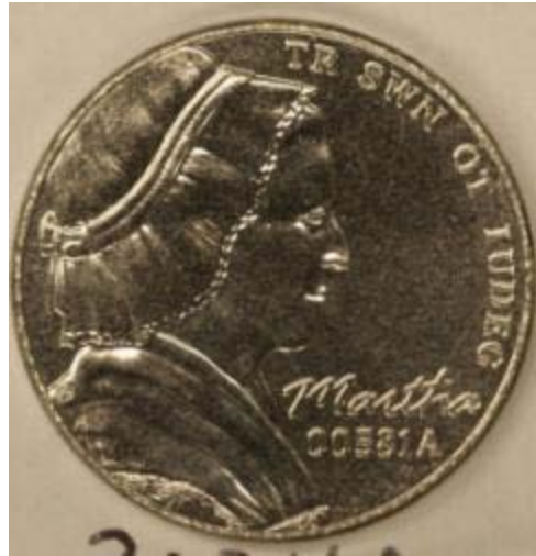
Figure 2-15. 302HQ stainless steel 5-cent nonsense piece struck at 70 tonnes.
