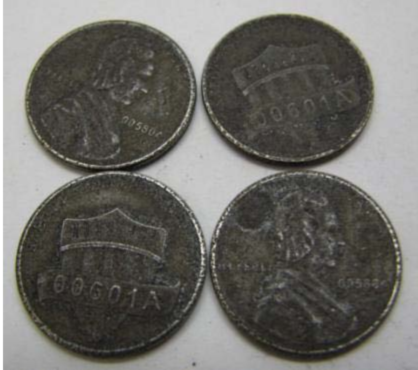
Figure 2-F-6. Wear tested aluminized steel (Ryerson) one-cent nonsense pieces.
