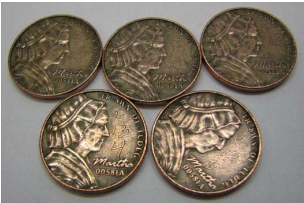
Figure 2-F-16. Wear tested nickel-plated 31157 5-cent nonsense pieces.
