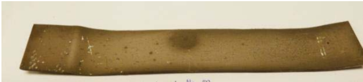
Figure 2-G-12. Carbonyl nickel-coated steel specimen bent back and forth several times.
