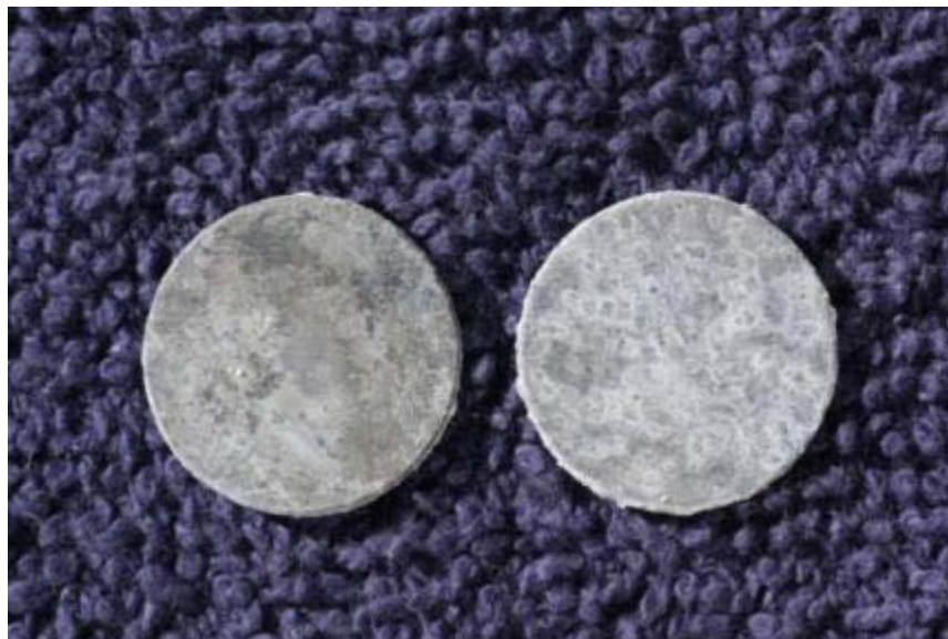
Figure 1-3. A190 planchets after 30-day atmospheric exposure during a rainy period.
