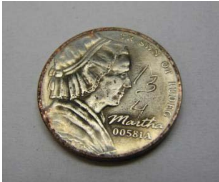
Figure 2-F-16. Wear tested nickel-plated 31157 5-cent nonsense pieces.
