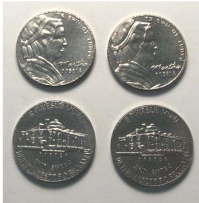
Figure 2-E-14. Steam corrosion tested 430 stainless steel 5-cent nonsense pieces.
