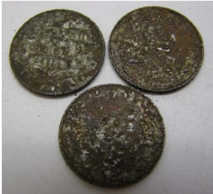
Figure 2-F-4. Wear tested 5052-H32 one-cent nonsense pieces.
