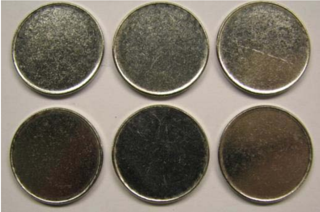
Untested, as-received on left, lightly sanded and tested in middle, and tested in ready-to-strike condition on right.
