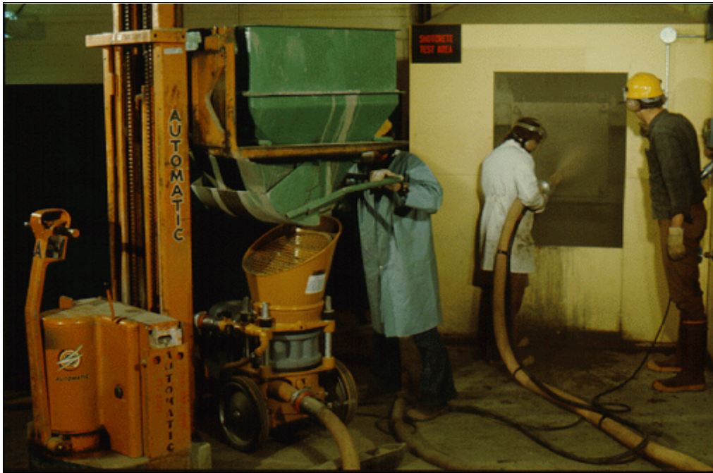
Figure 43.—Dry mix shotcrete equipment being used in the Denver concrete laboratories.
