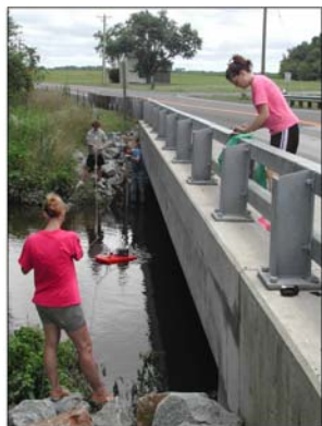
Stream gauging activities using an acoustic doppler current profiler
