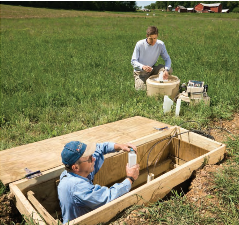
Tony Buda (right) and laboratory worker David Otto collect runoff water samples from a hillslope trench that is being used to monitor lateral subsurface flow pathways during and after storms.
