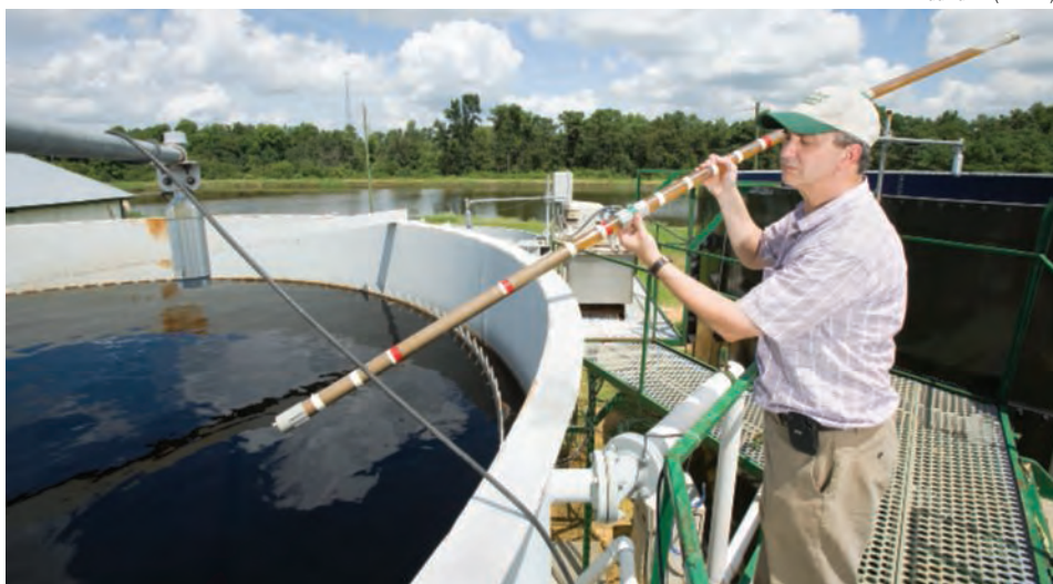
Using a deep sampling probe, Ariel Szogi inspects the amount of calcium phosphate produced in a phosphorus-separation module that is part of the new system.
