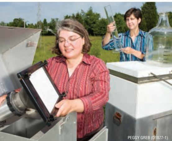
Chemists Cathleen Hapeman (left) and Laura McConnell use air and rain sample collection devices to study the fate of atmospheric pollutants in the Chesapeake Bay region.
