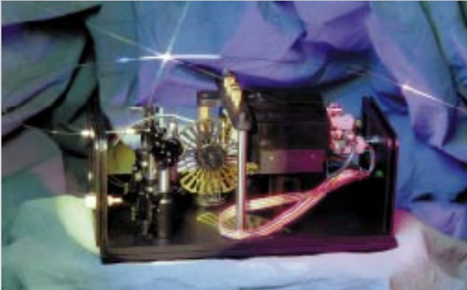
Figure 2. Livermore's temperature feedback system, including the award-winning sensor. A two-color infrared temperature sensor controls the laser used to heat the weld site.
