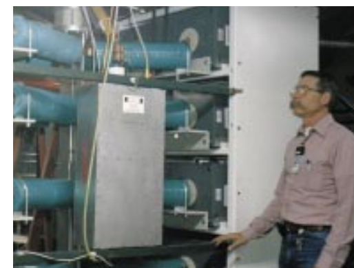
Figure 7. NIF's 1.7-megajoule power conditioning modules, each housing 20 advanced capacitors, are being tested by Sandia National Laboratories, Albuquerque.
