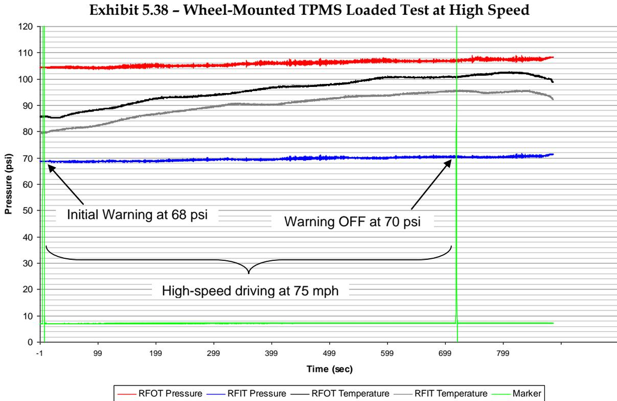
As shown in Exhibit 5.38, the wheel-mounted TPMS also exhibited increased pressure effects due to tire heating, but the warning indication was discontinued once the pressure reached the warning threshold.
