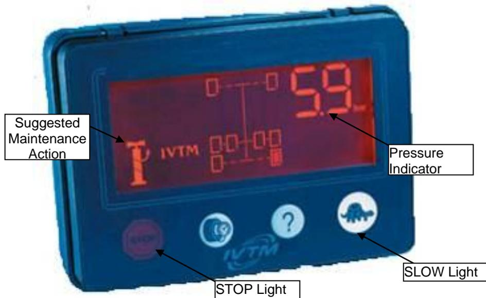
The test drivers commented that the interface in Exhibit 5.47 for the IVTM was difficult to read in the daytime. The black and red display, in addition to the “STOP” and “SLOW” lights, was not
