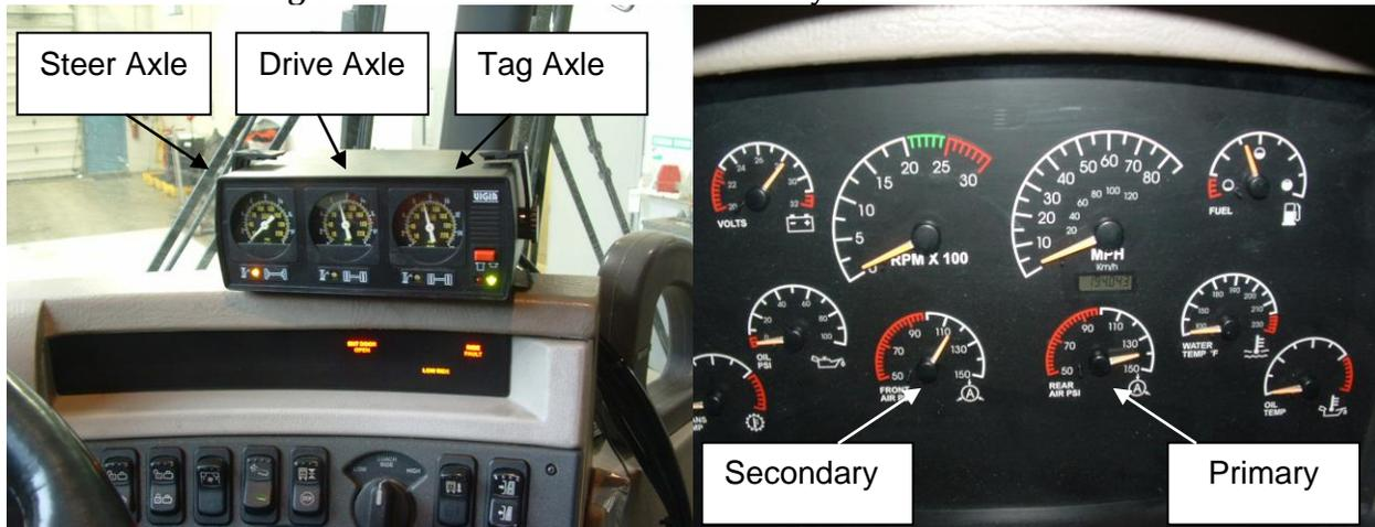
Vigia CIS Disablement Mode 2 differed from Mode 1 in that the quick disconnect sealed off the line from the console. The hose check valve protected the RFS tire from deflation. The system indicated normal pressure in the LFS tire and functioned normally, but it could only inflate the LFS tire.
