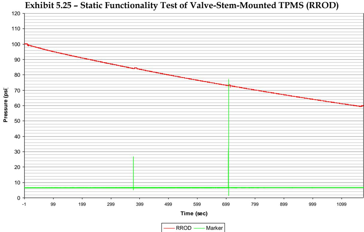
For this system, Exhibit 5.25 shows that an initial leak rate of 1.5 psi/minute on the RROD resulted in the initial warning indicating at 84 psi and a second warning indicating at 72 psi, as shown by the Marker channel. These readings generally correspond to the manufacturer's specification of an initial warning indicator at 12.5 percent below CIP (87.5 psi for our test) and a second indicator at 25 percent below CIP (75 psi for our test).
