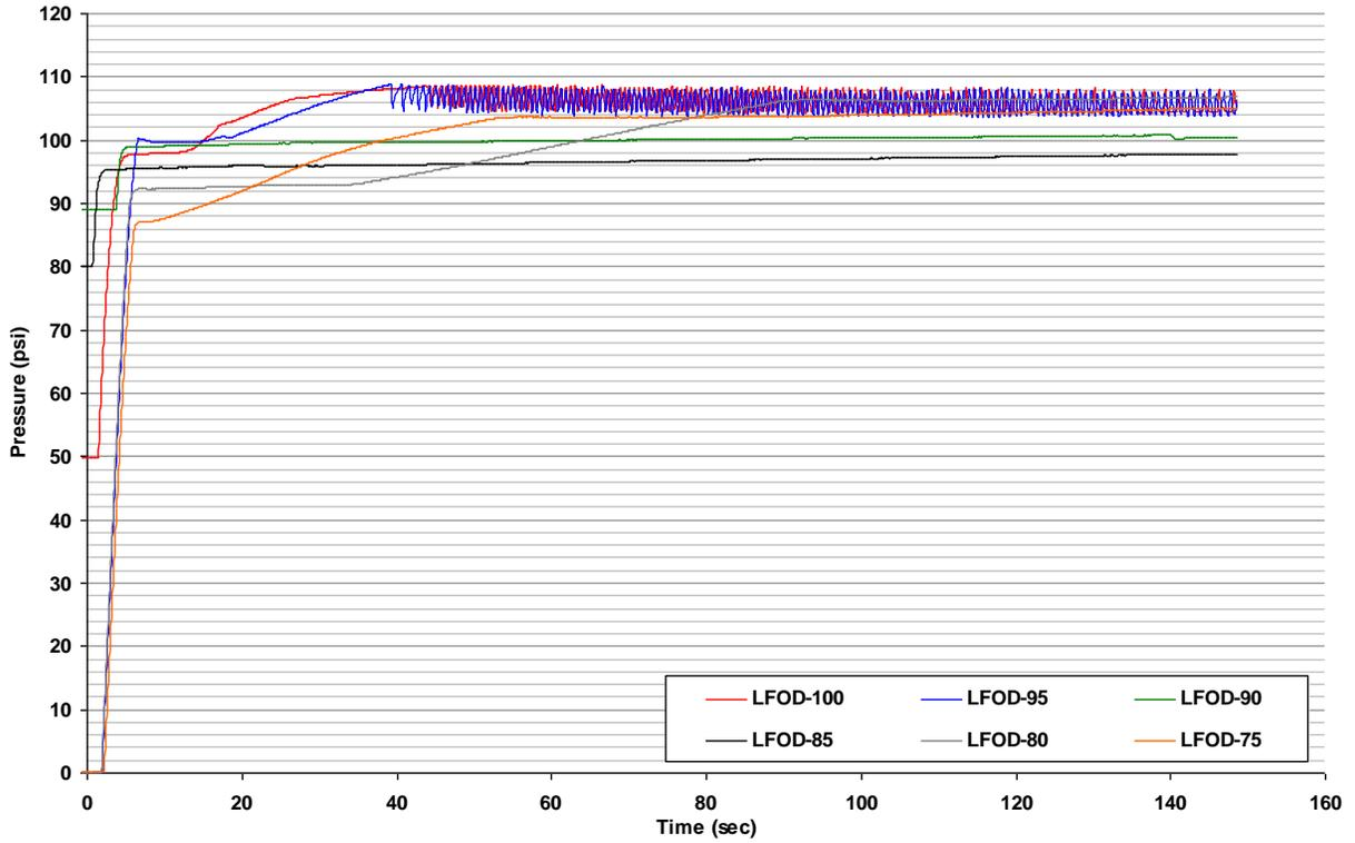
Exhibit 5.58 shows the static functionality test of the PSI CIS.
