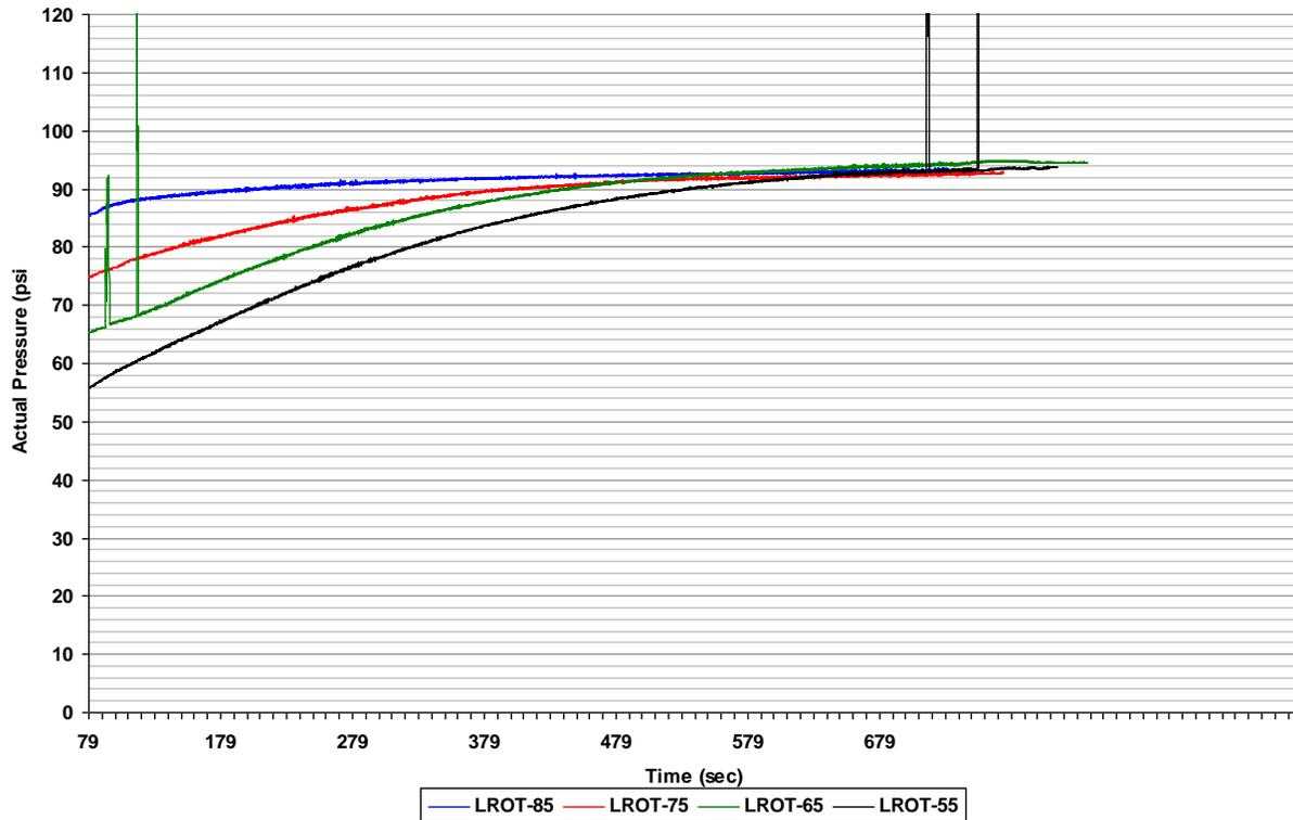
As shown in Exhibit 5.60, the PSI CIS performed similarly under the dynamic test as it did under the static test – inflating tires (from 86, 73, 63 psi) up to 93 to 95 psi. The spikes in the LROT-65 trace are due to noise in the data. These same test series were performed on the RFIT tire, which experienced similar test results as shown in Exhibit 5.61.
