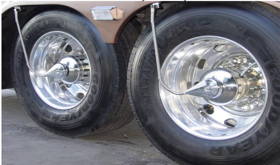
An alternative approach, used by Arvin Meritor, uses the axle to deliver air to the wheel with the rotary union located in the hubcap at each wheel end, as shown in Exhibit 1.4.
