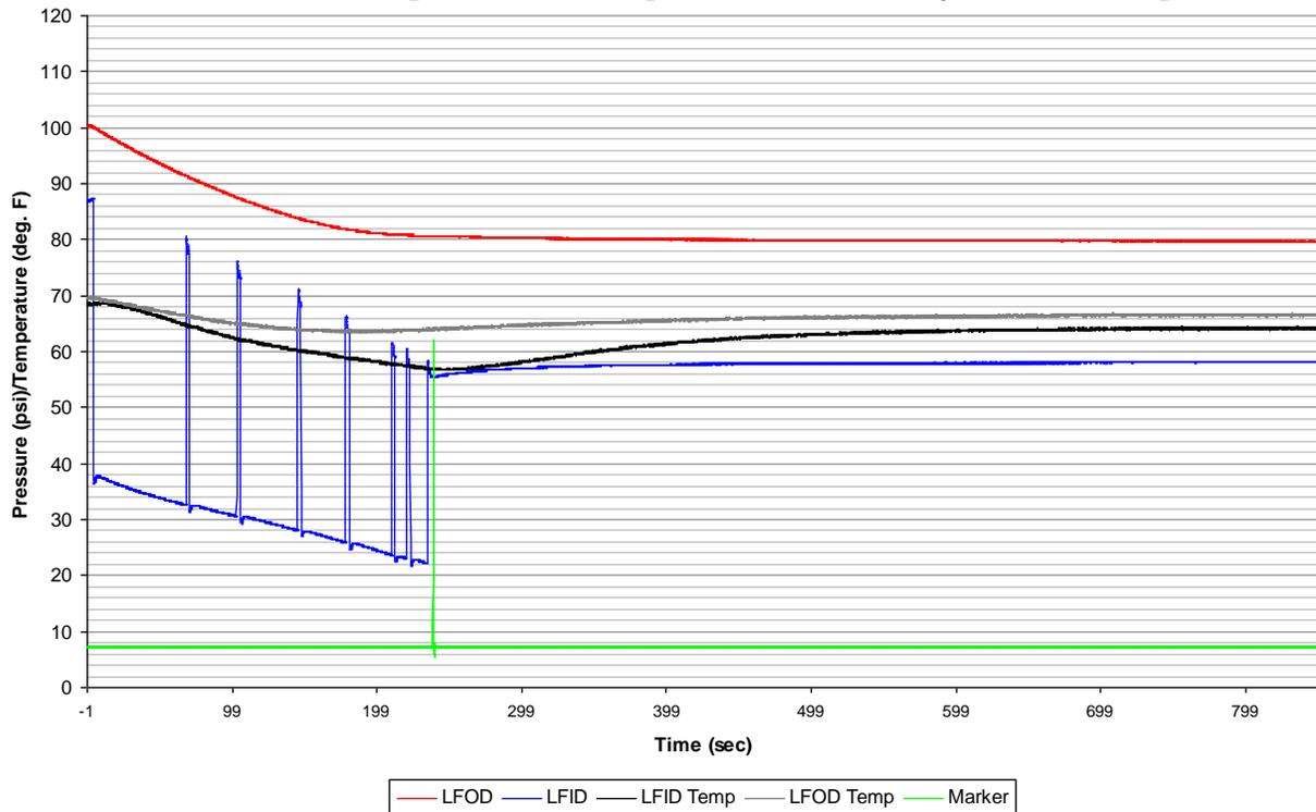
Exhibit 5.4 summarizes the data from the Link equalizer static functionality testing. The system appears to equalize the pressure of the tire experiencing air loss until it decreases to approximately 80 psi. When a leaking tire deflates below 80 psi, the system will stop pressure equalization when the pressure of the intact tire reaches 80 psi to prevent the total loss of pressure in both tires of a dual installation.
