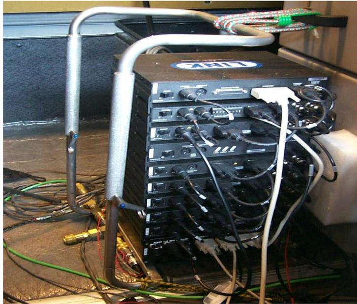
The system is modular and, for this test program, was configured with eight multi-channel signal-processing modules. See Exhibit 3.13 for complete specifications.
