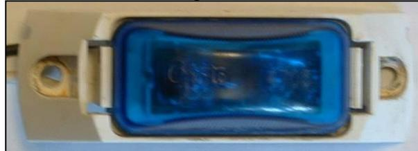
As shown in Exhibit 5.81, the PSI CIS relies on a simple trailer-only blue indicator light. The light should be mounted in such a way as to allow the vehicle operator to see it through the left-side mirrors. In the test setup, the indicator light did not function consistently and the manufacturer representative present could not find the source of the fault.
