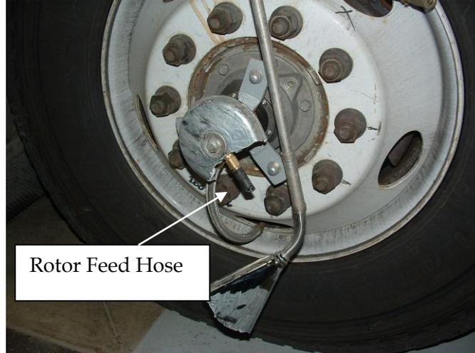
Vigia CIS Disablement Mode 5 was, in effect, similar to Mode 2. The RFS down pipe was disconnected from the system at the rotor and at the quick disconnect. The RFS and LFS tires were protected by check valves, and the RFS circuit was isolated from the system by the quick disconnect. The console indicated 105 psi and functioned normally, but was only monitoring the LFS tire.
