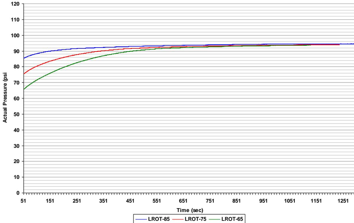
As shown in Exhibit 5.58, the PSI CIS inflates under-inflated tires (from 85, 75, and 65 psi) up to 94 to 95 psi, which was the system pressure set by the manufacturer’s installers who outfitted the test trailer. This is as expected based upon the intended functionality of the system and the system pressure setting set by the manufacturer. The same test series was performed for this system on the RFIT tire, which exhibited similar results within a 2- to 3-psi range, as shown in Exhibit 5.59.
