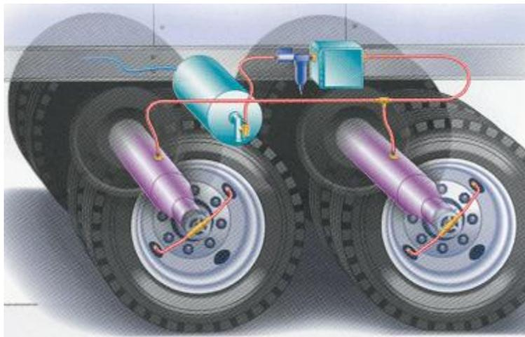
Central tire inflation systems can supply air to the tires either on demand via a manual request by the driver, or automatically triggered through sensors that monitor tire pressure. Central tire inflation systems can be broken down into two types – constant and variable.
