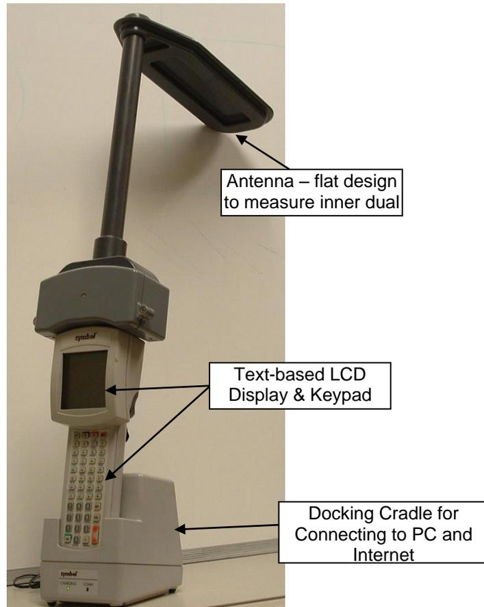
The technicians and test engineers found the handheld reader cumbersome in operation and required a significant learning curve to use. The software was text-based and the data entry from the handheld unit required that its cradle be connected to a computer with Internet access.
