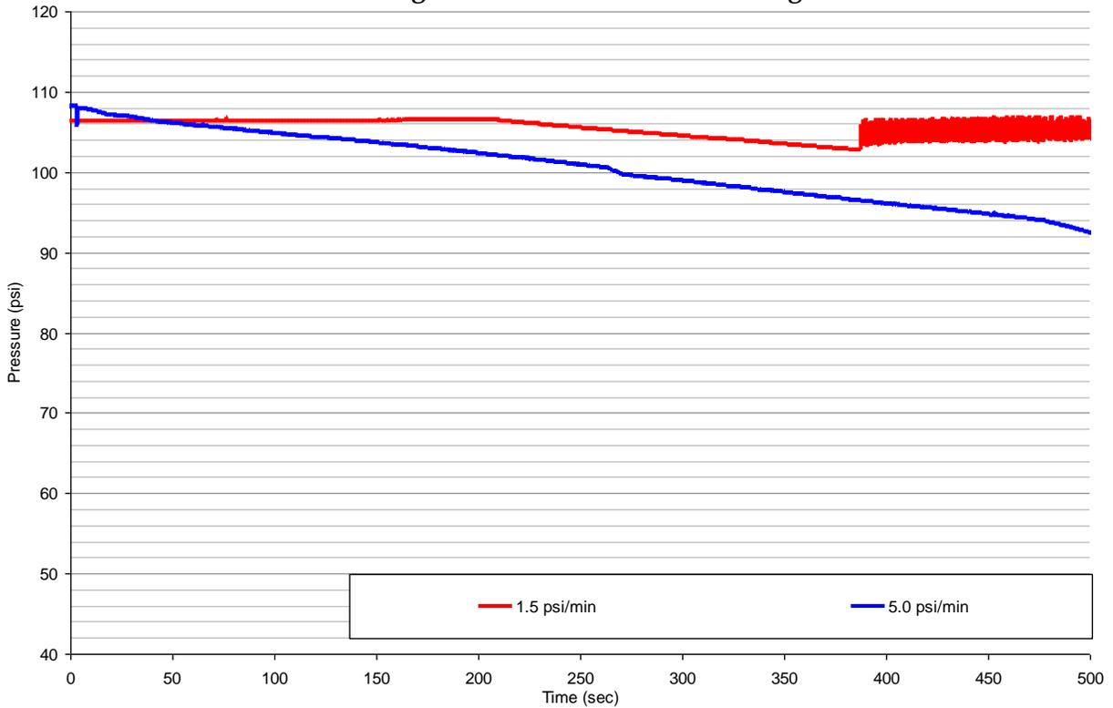
Exhibit 5.65 shows the threshold warning level test of the PSI CIS.
