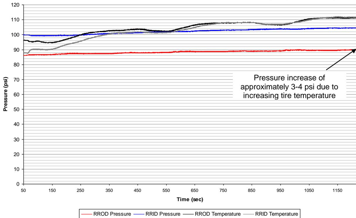
To accommodate this effect, some TPMS measure the tire temperature and compensate for the increased pressure by calculating an equivalent CIP. This test is designed to determine, for the TPMS technologies selected for testing here, whether they compensate for the increased pressure as a result of sustained high-speed driving. Exhibit 5.35 shows the general test procedures performed.
