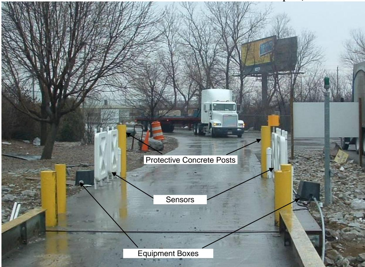
In Exhibit 5.51, the gate reader sensors are protected by concrete posts to prevent accidental damage by vehicles. The eTire TPMS tested used a passive tire tag (i.e., the tag was not powered, but received its power from the measuring sensor), which resulted in a very short transmission
