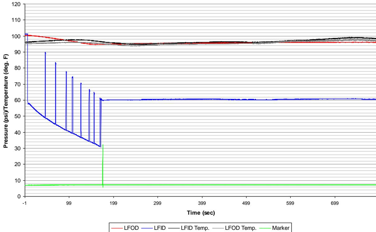
Exhibit 5.18 summarizes the data from the Link equalizer failure mode testing. During the static and dynamic testing with a rapidly leaking tire, the system appears to equalize pressures down to approximately 80 psi in the LFID/LFOD and RFIT/RFOT tire pairs. The RROD/RRID and LROT/LRIT pairs, however, stopped equalizing when the pressures of the isolated tires were in the high-80s psi range.
