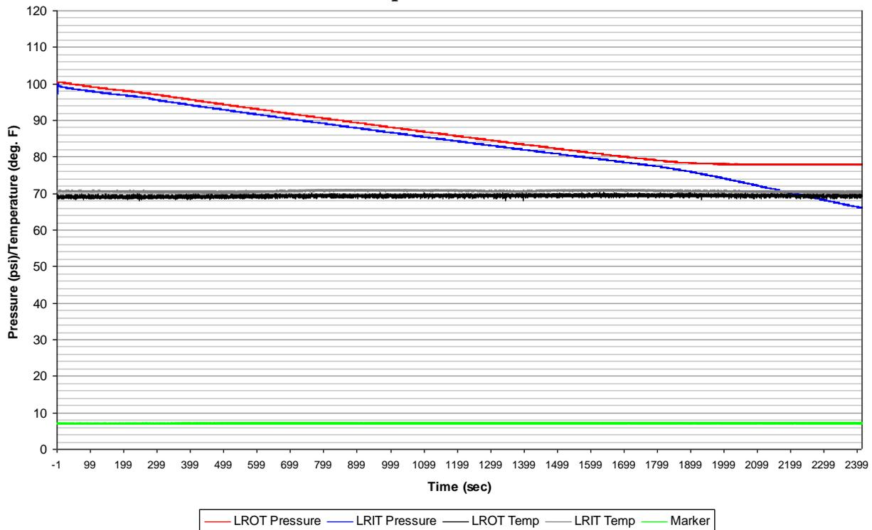
Exhibit 5.12 shows the Link equalizer equalizing a dual installation during a dynamic test at 45 mph. Here, the LRIT tire's pressure slowly dropped due to an induced leak of approximately 1.5 psi per minute, while the corresponding initial LROT was set at 100 psi. The tires begin to equalize immediately on the reduction of pressure as evidenced by both the LRIT and LROT traces. The data show that the LROT tire stabilized at approximately 75 psi, while the LRIT tire
