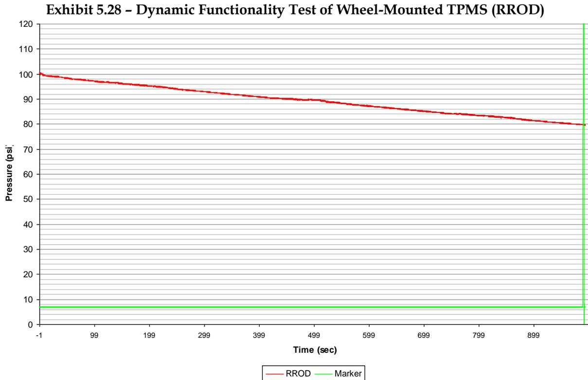
In general, each system tested, valve- or wheel-mounted, had the base-level functionality expected based on their individual designs. All provided warnings, although the deviation from the expected warning pressure varied from system to system and tire to tire given a slow leak (approximately 1.5 psi/min initial rate). The exact deviations from the expected warning thresholds were tested and analyzed in the warning threshold level tests in the next section.
