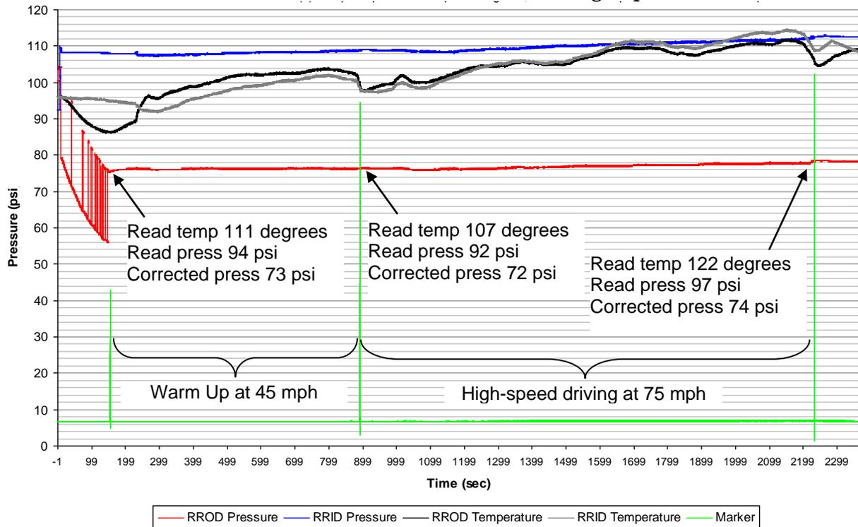
In Exhibit 5.40, the handheld reader recorded the temperature read by the sensor, the pressure read by the sensor, and the corrected pressure as a result of the sensor compensating for the temperature inside the tire. Exhibit 5.40 shows that the eTire TPMS sensor compensated for the increased temperature and pressure due to sustained high-speed driving. Exhibit 5.41 show the results of each of the tests for the tire-mounted TPMS.
