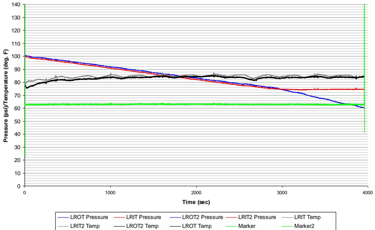
Exhibit 5.13 summarizes the data from the Link equalizer threshold warning testing. During the static and dynamic testing with a slowly leaking tire, the system appears to equalize pressures down to approximately 80 psi, although the pressures of the isolated tires were in the mid to upper 70 psi range. Because the air loss rates were low, the equalizers on the RROD/RRID and LFID/LFOD equalized but did not isolate the intact tire of the dual pair during the test period.
