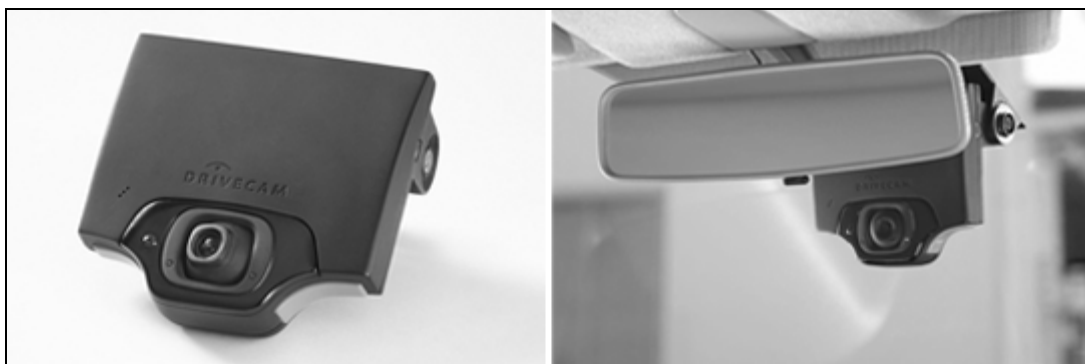
Figure 1. Photo. Event recorder (left) and typical installation of event recorder behind the vehicle's rearview mirror (right).
