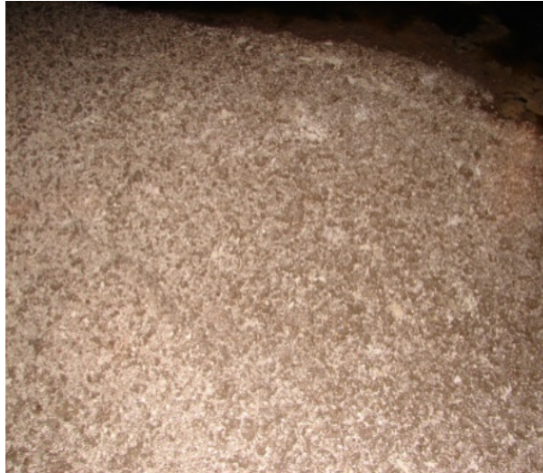
Figure 2.2-2. This picture was taken at the bottom of S1. The white material is presumed to be the flake material that exited the stack on September 10 th and 18 th .
