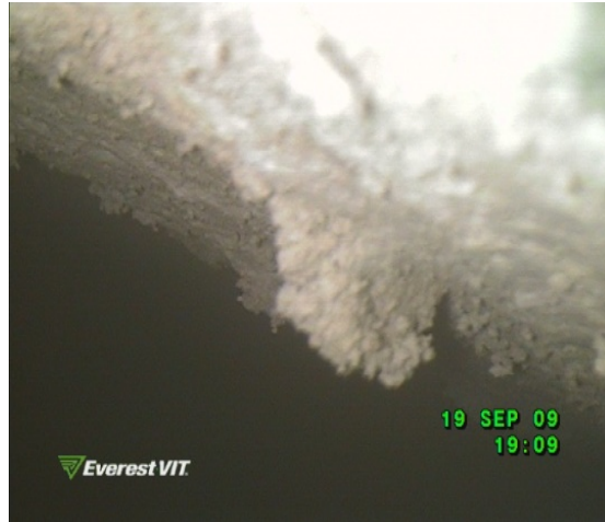
Figure 2.2-1. This picture was taken with a borescope of S1 at the 330 foot elevation. A similar inspection of S2 showed no such buildup.
