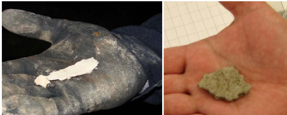
Figure 2.2-5. This is a picture of the two types of material found on the stack liner and on the stack floor. The material on the left is the light friable material while the picture on the right is the more dense buildup.
