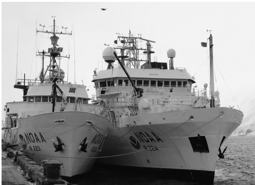
Figure 1. The NOAA ships Miller Freeman (left) and Oscar Dyson (right) in Dutch Harbor, Alaska. Although the ships are of similar length, the Dyson has approximately 30% more displacement and approximately 40% more horsepower. Photo by Alex De Robertis.
