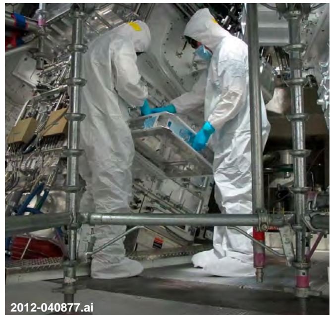
Figure 4-5: Two facility workers in PPE are exchanging a potentially contaminated optic from the final optics assembly attached to the NIF target chamber.
