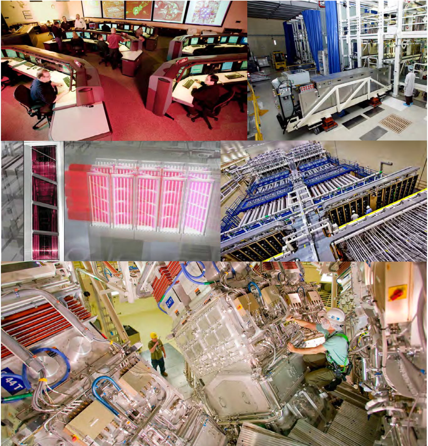
Figure 1-3: Images of NIF. Clockwise from upper left: NIF control room. A preamplifier module installed as an LRU. One of NIF's two identical laser bays. Maintenance on a NIF beamtube in the target bay. NIF laser glass cassettes holding amplifier slabs.
