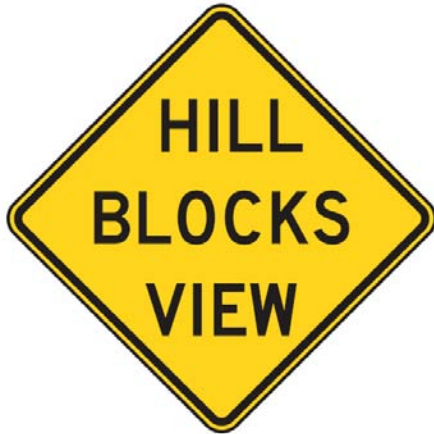
FIGURE 57 Sign for crest vertical curve with inadequate stopping sight distance.
