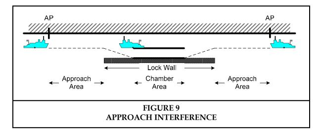
For purposes of simulation, it is necessary to associate this with a description of the location of a vessel within the internal geometry of a lock. It is necessary to provide such a description to understand how these four time increments are specified exactly, and how they relate to movements of a vessel.
