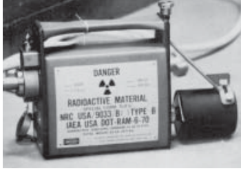
Portable radiography camera used to test for cracks in metal
