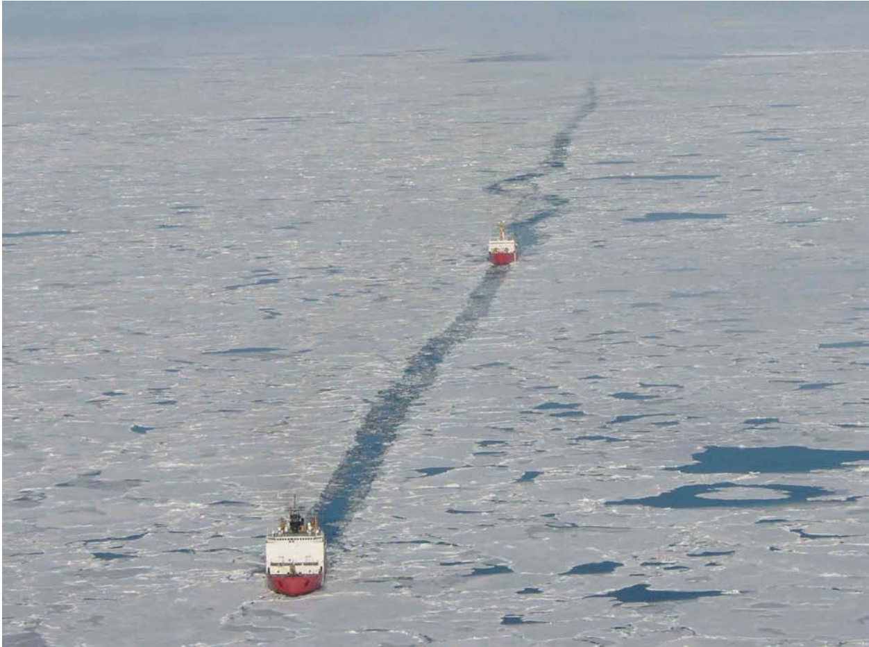
FIGURE ADD-1. Icebreakers Healy and Louis S. St-Laurent transiting 10/10 ice pack on 2 September 2009, showing minimal disturbance to the ice pack abeam of the ship's path, small jog to avoid larger ice body, and closing of the pack ice in the ship wake.
