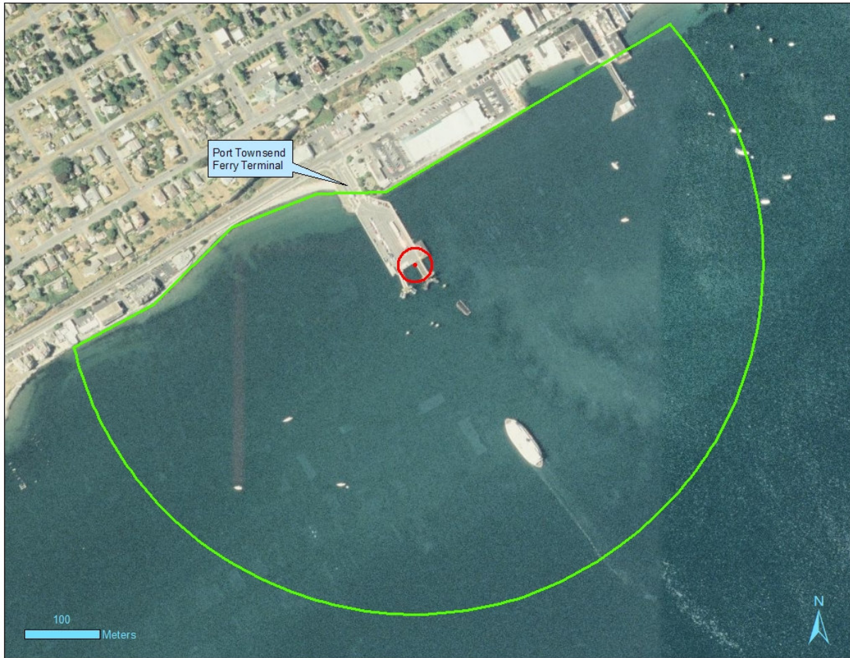
Figure 2 – Approximate 22 m (red circle) impact pile driving shut-down safety zone and 464 m (green) Level B acoustical harassment ZOI.
