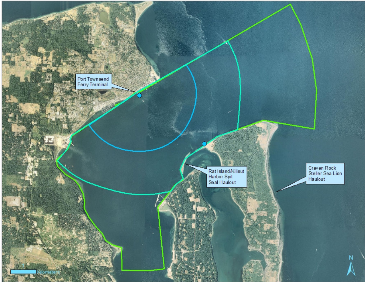
Figure 5 – Vibratory timber pile removal 2.2 km ZOI (blue line) and marine mammal monitoring locations (blue circles).
