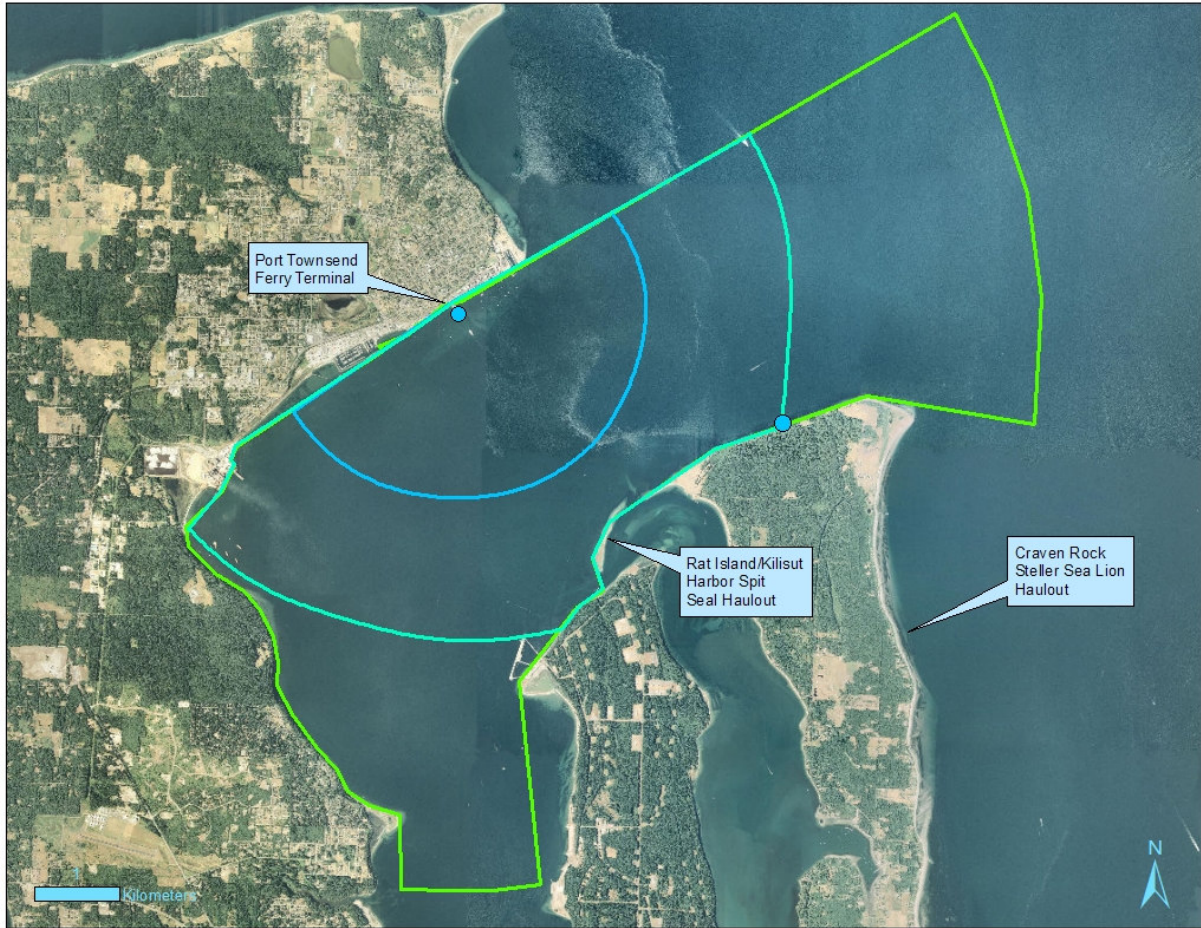
Figure 6 – Vibratory 24” steel pile removal 4.0 km ZOI (turquoise line) and marine mammal monitoring locations (blue circles).
