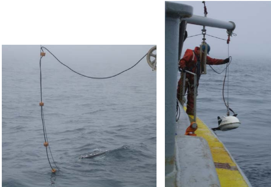
Figure 3.7. Dual Frequency Bubble Pulser (left) and Datasonics Chirp II (right).
