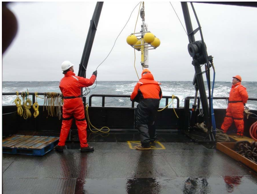
Figure 3.1: OBH system being deployed from the Norseman II .
