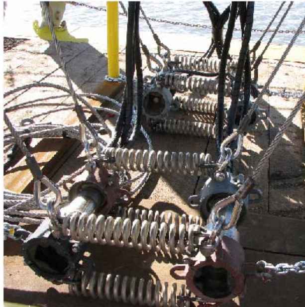
Figure 3.6. GEO LLC two gun array.
