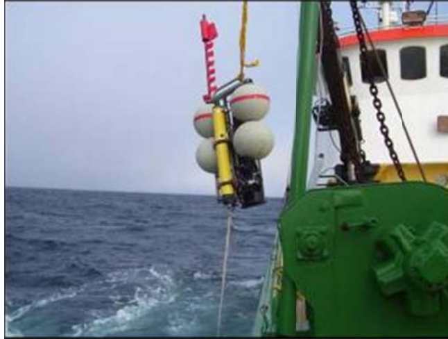
Figure 2. Hydrophone recording system being deployed at sea. The hydrophone system is an autonomous recorder with very high recording resolution. Acoustic data is stored internally on a hard-drive.
