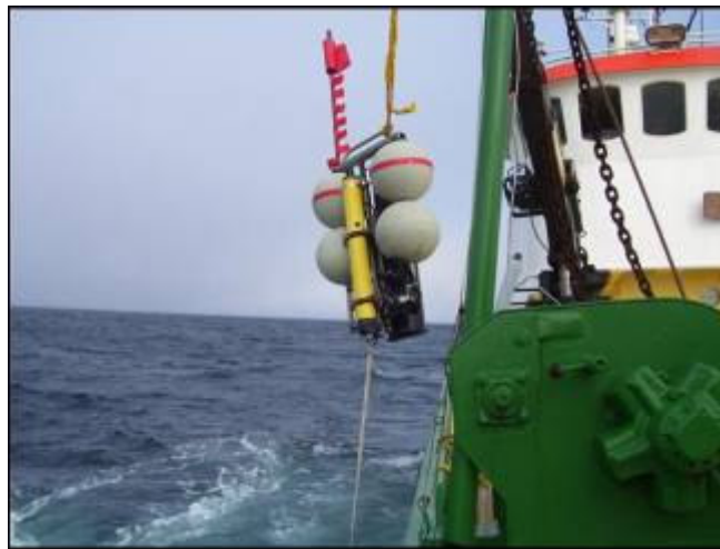
Figure 3. Hydrophone recording system being deployed at sea. The hydrophone system is an autonomous recorder with very high recording resolution. Acoustic data is stored internally on a hard-drive.
