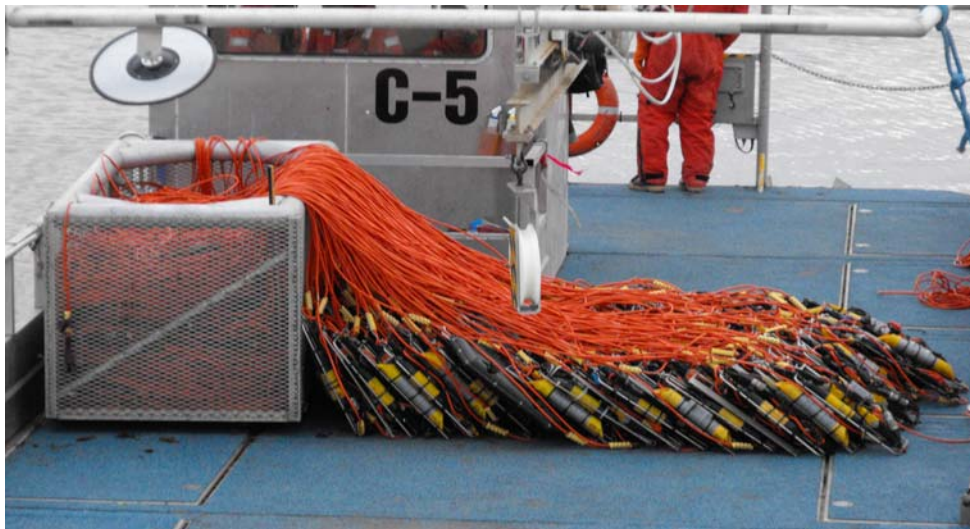
FIGURE C.14. An example of ocean-bottom cables being prepared for deployment. Hydro- and geophone stations are attached to the cables (laying on the vessel deck).
