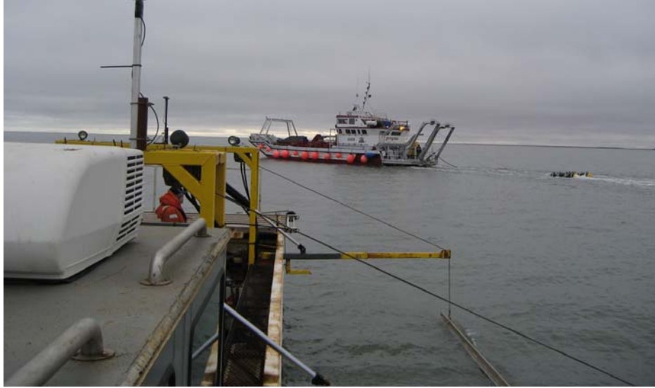
FIGURE C.10. Photo from the Shirley V showing starboard side placement of the airgun array (in the foreground) versus the stern towed placement of the airgun array on the Peregrine (in the background) used during the Eni/PGS seismic survey.
