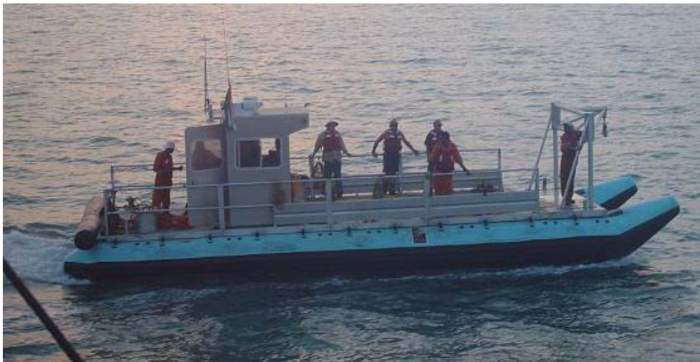
FIGURE C.11. An example of a cable DIB vessel used during the Eni/PGS seismic survey.
