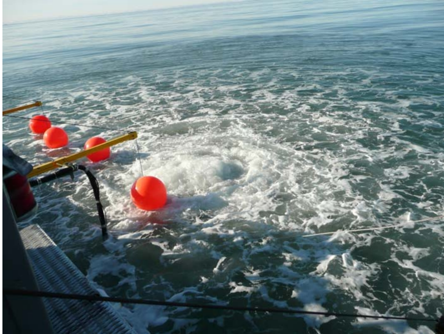
FIGURE C.6. Placement location of (half) of the airgun array from the Wiley Gunner or Shirley V used during the Eni/PGS seismic survey.
