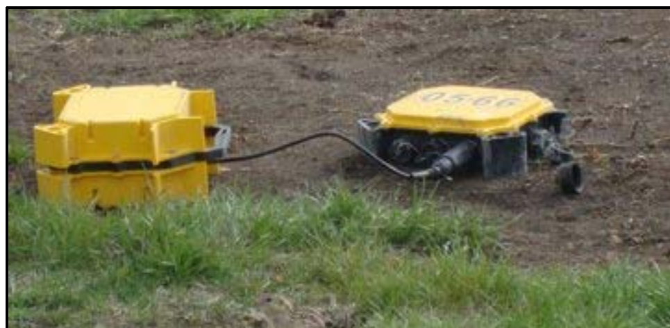
Figure 8. Typical Wireless Iseis Sigma Nodal Land Recording System Installation (Battery Pack is located on the left and Recording System on Right)
