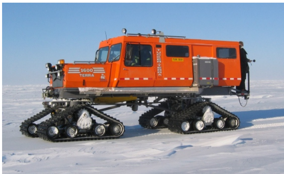
FIGURE 1.4. Tucker tracked vehicle powered by a Cummins 6-Qsb 173 HP diesel engine.
