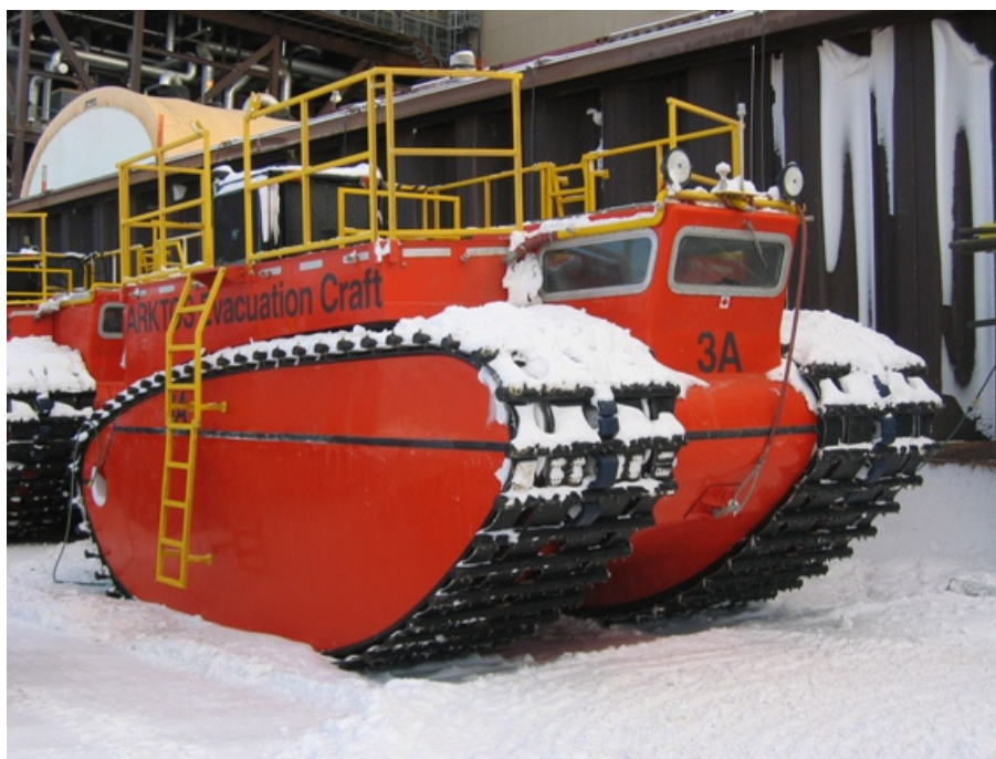
FIGURE 1.7. Articulated ARKTOS evacuation craft used as Northstar's emergency escape vehicles.
