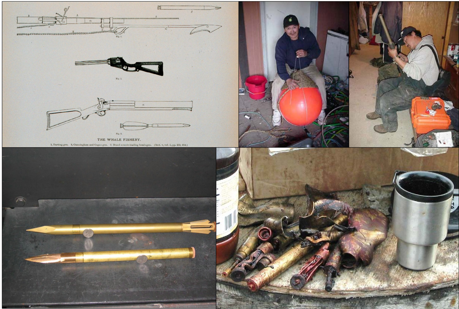
FIGURE 3.1. Subsistence whaling equipment. Top left to right: NOAA archive illustration of darting gun (above) and shoulder gun (center and below); wrapping rope on float (to attach to darting gun); and cleaning shoulder gun. Below: Unloaded new whale bombs (quarters for scale); and some fragments of exploded bombs recovered from whales.
