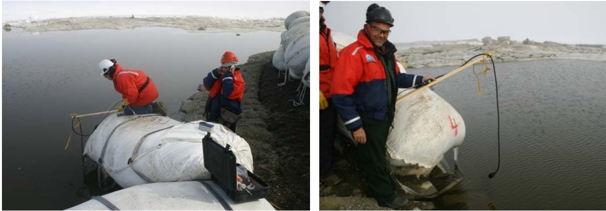
FIGURE 2.5. Listening for pops with the cabled hydrophone deployed in the moat along the western shore of Northstar, 11 June 2009.
