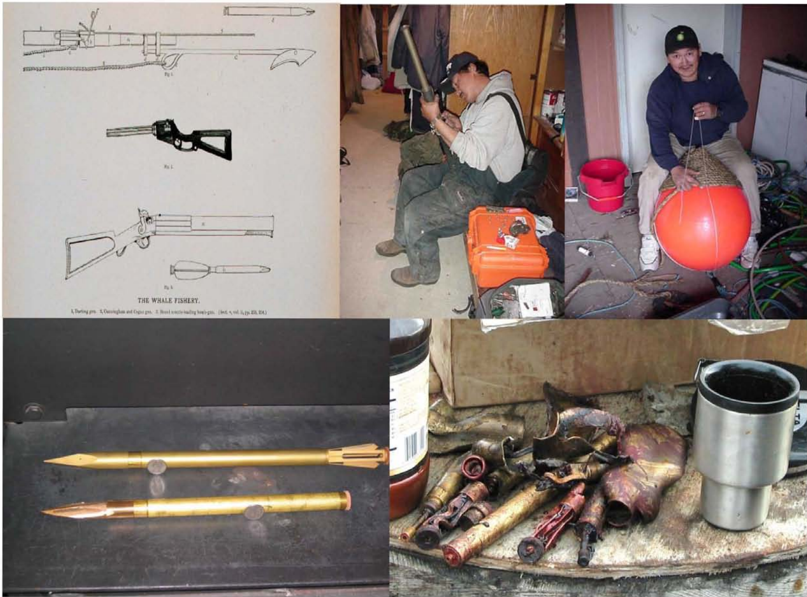
FIGURE 5.1. Left to right, top to bottom: NOAA archive photo showing whaling gear, cleaning shoulder gun, wrapping rope on float (to attach to darting gun), unloaded new whale bombs (quarter for scale), some fragments of exploded bombs recovered from whales.
