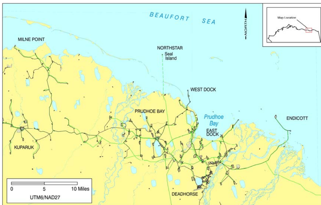
FIGURE 1.1. Location of the Northstar Development at Seal Island in the central Alaskan Beaufort Sea. Seal Island was an artificial gravel island constructed for exploration drilling in the 1980s. Northstar facilities were built on the eroded remnants of Seal Island in 2000.
