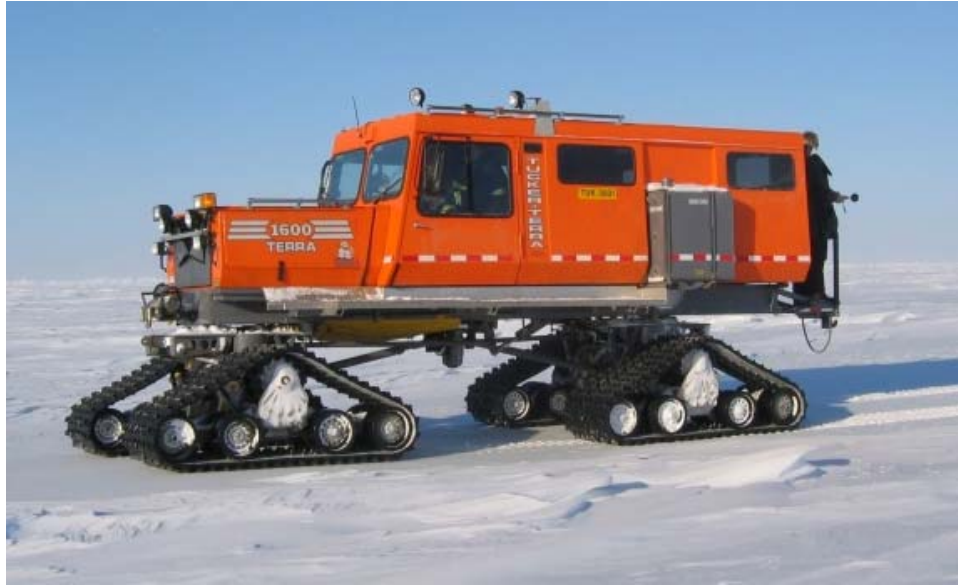
FIGURE 1.4. Tucker tracked vehicle. Power is from a Cummins 6-Qsb 173 hp diesel engine; weight of the Tucker ranges between ~4536 and 7257 kg (10,000 – 16,000 lbs).
