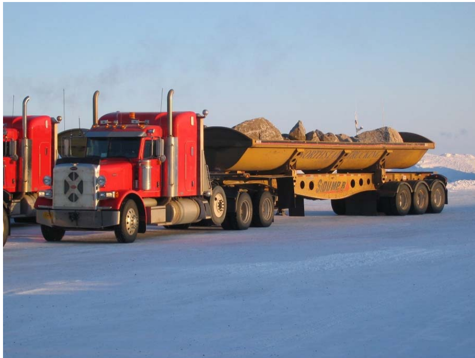
FIGURE A1. Side-dump trucks used to transport boulders.
