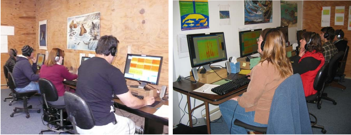
FIGURE 2.7. Eight of the 21 work stations at Greeneridge Sciences where analysts identify and localize whale calls. In the left picture, note 10 spectrograms on the screen of the closest analyst, representing the 10 DASAR locations of the Northstar offshore array.
