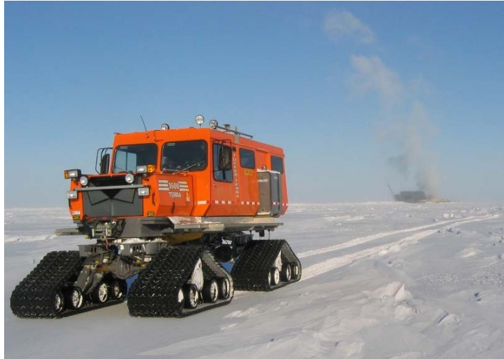
FIGURE 1.4. Tucker tracked vehicle. Power is from a Cummins 6-Qsb 173hp diesel engine; weight of the Tucker ranges between ~4536 and 7257 kg (10,000 – 16,000 lbs).
