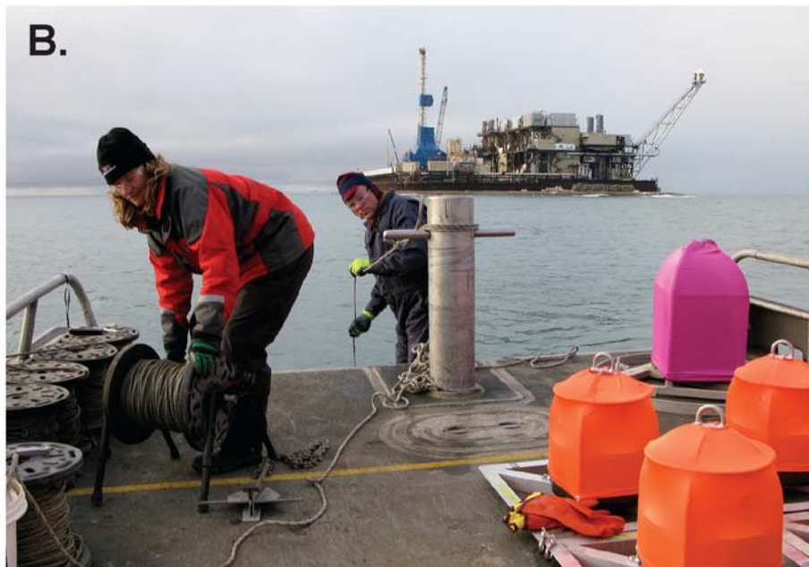
FIGURE 2.1. DASAR recorders. (A) Schematic diagram of the components of the DASAR-C08 recorder. (B) DASARs on the back deck of the ACS vessel Mikkelsen Bay , with Northstar in the background. The three DASARs that are closest to the photographer are DASAR-C08 recorders, whereas the recorder farthest back on the deck is a DASAR-A. The near-island DASAR NSa is being lowered to the seafloor with the lowering line (tied to the davit) by ACS deck supervisor Mark Stopha. LGL scientist Lisanne Aerts is readying the spool of ground line, which is connected to the DASAR and is to be laid out on the seafloor in the next step of the deployment.
