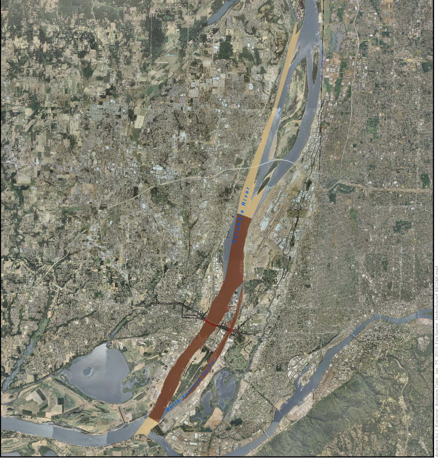
Figure B-5. Extent of underwater vibratory pile-driving noise exceeding 120 dB RMS disturbance threshold for pinnipeds.
