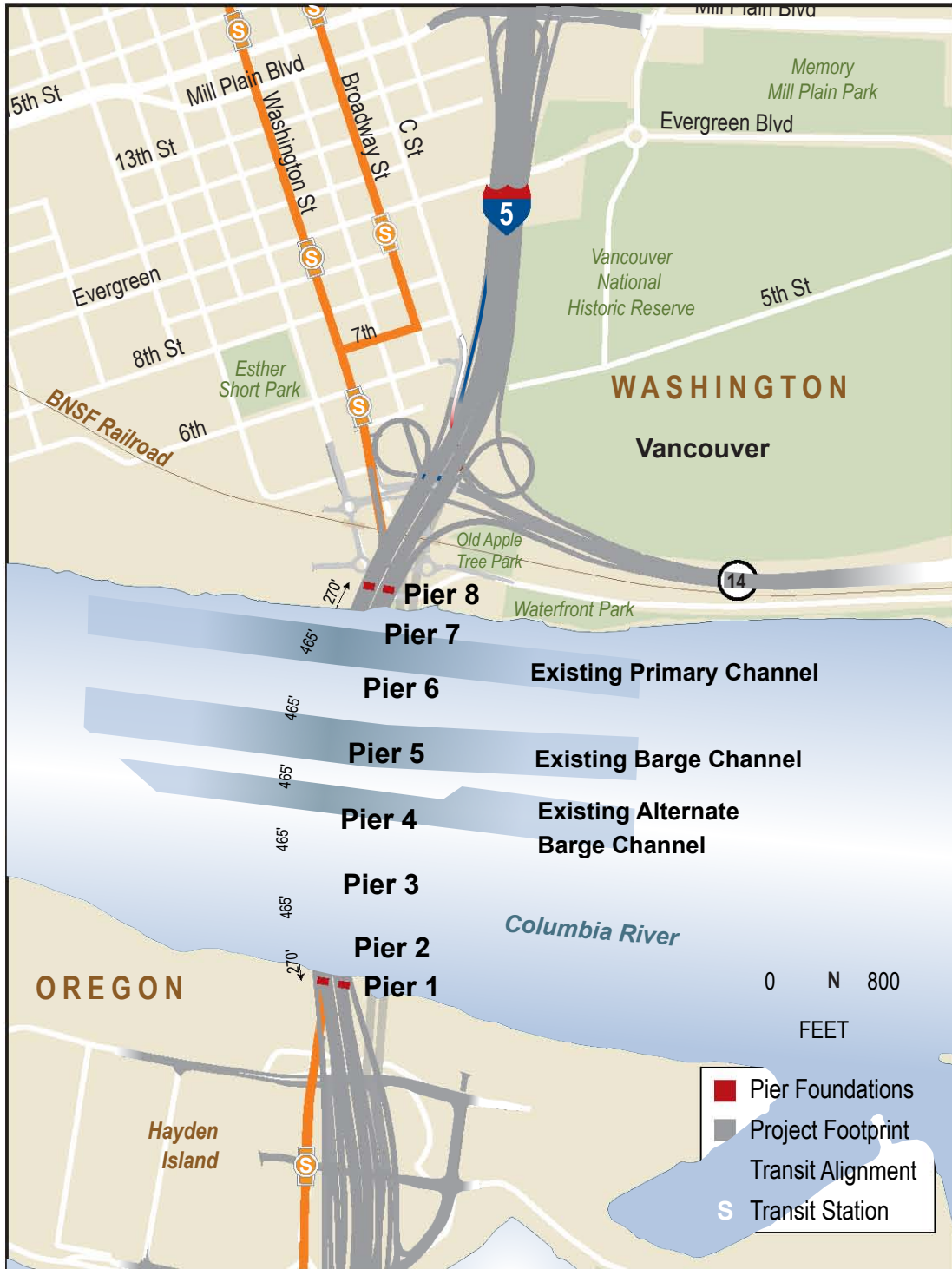
Figure 1-2. Proposed Layout of Columbia River Bridge Showing Piers and Existing Navigation Channels
