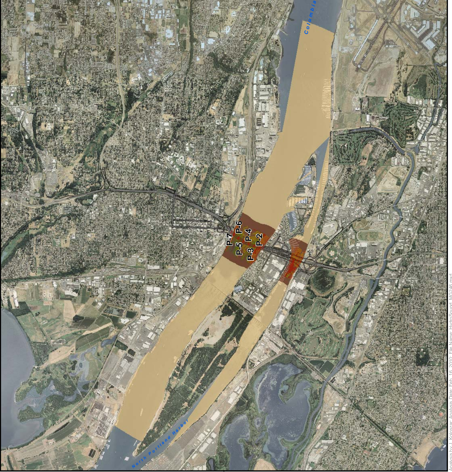
Figure B-4. Extent of underwater impact pile-driving noise exceeding 160 dB RMS disturbance threshold for pinnipeds, 36 to 48-inch pile
