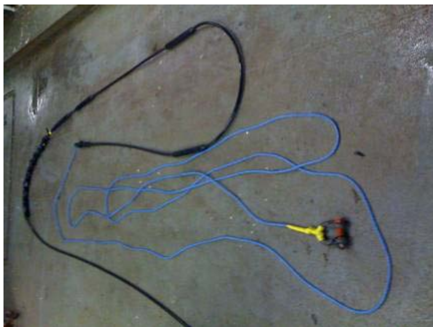
Figure 28 Rope drogue and first chain weight secured near hydrophone elements.
