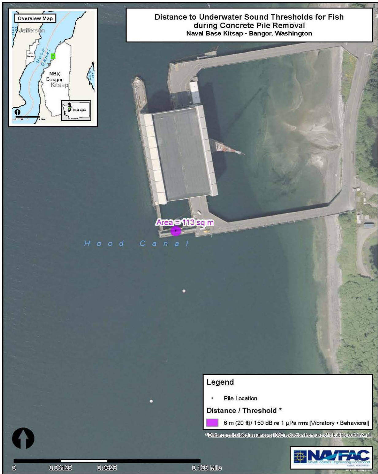
Figure 3-14 Distance to NMFS Underwater Noise Threshold from Utilizing a Chipping Hammer During Concrete Pile Removal
