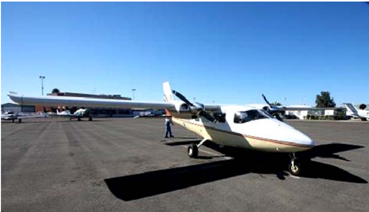
Figure 1. The Partenavia P68-C fixed-wing, twin-engine aircraft used during the aerial survey monitoring.
