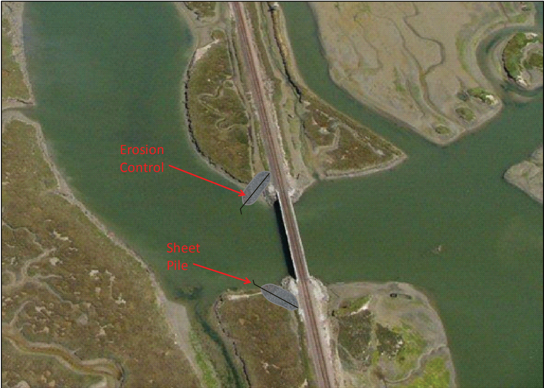
Representative of visible portion of the sill structure, as seen from an aerial perspective, at mean low tide. Approximately 170 feet of sheetpile and erosion protection represented.
