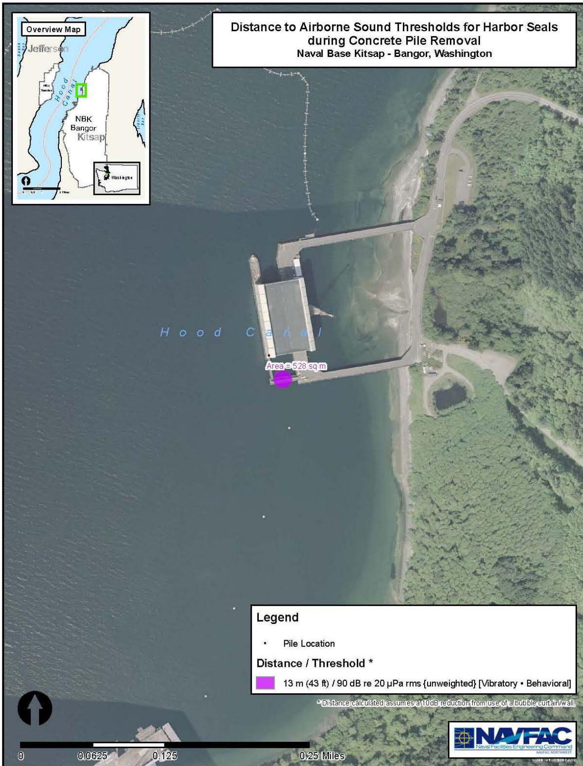
Figure 6-10 Distance(s) (m) to Airborne Sound Thresholds for Harbor Seals from a Chipping Hammer During Concrete Pile Removal
