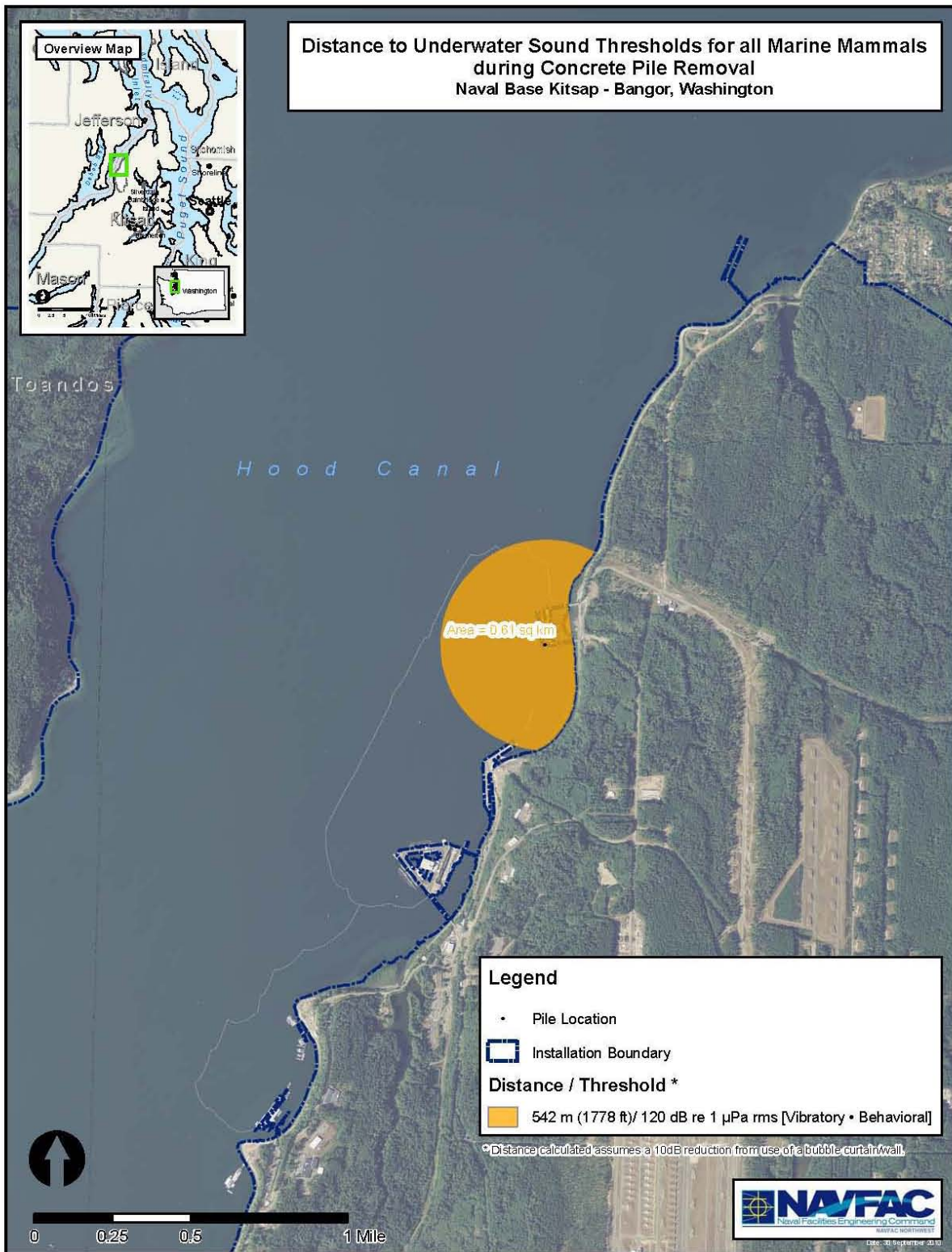
Figure 6-4 Distance(s) (m) to Underwater Sound Thresholds for all Marine Mammals from a Chipping Hammer During Concrete Pile Removal
