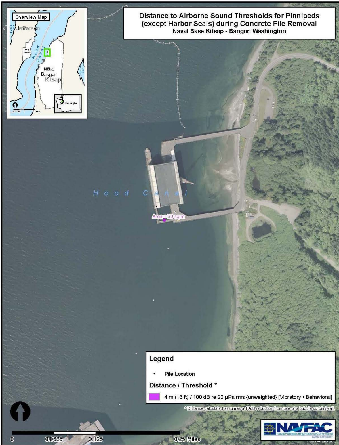
Figure 6-9 Distance(s) (m) to Airborne Sound Thresholds for Pinnipeds (except Harbor Seals) from a Chipping Hammer During Concrete Pile Removal
