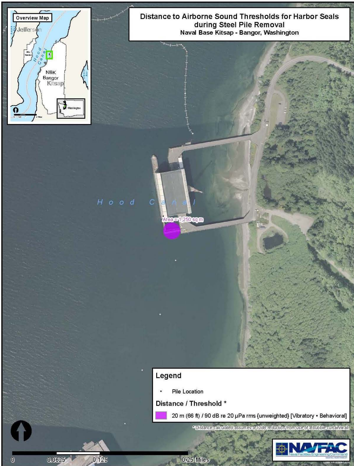
Figure 6-8 Distance(s) (m) to Airborne Sound Thresholds for Harbor Seals from Vibratory Pile Driving During Steel Pile Removal
