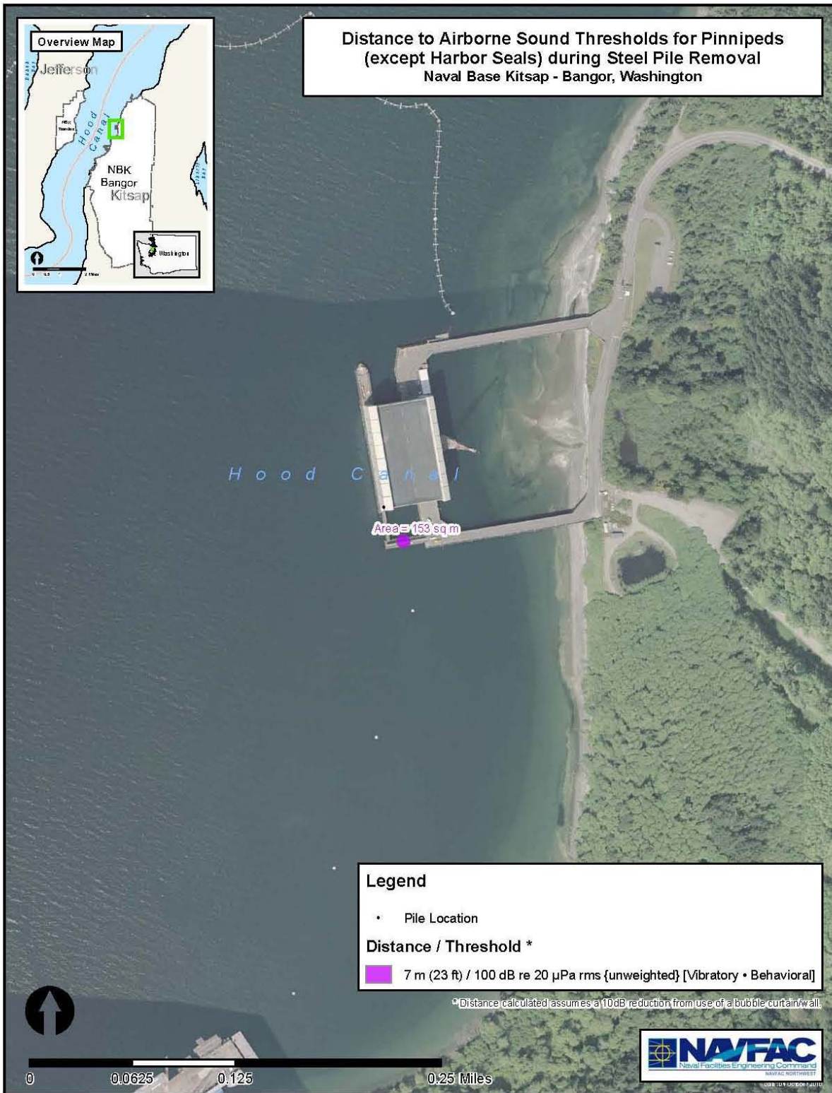
Figure 6-7 Distance(s) (m) to Airborne Sound Thresholds for Pinnipeds (except Harbor Seals) from Vibratory Pile Driving During Steel Pile Removal
