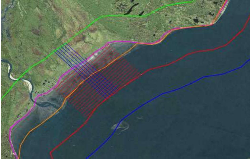
Figure 5. A Single Intertidal Patch, Six Lines of Nodes (Blue), 16 Source Lines (Red).
