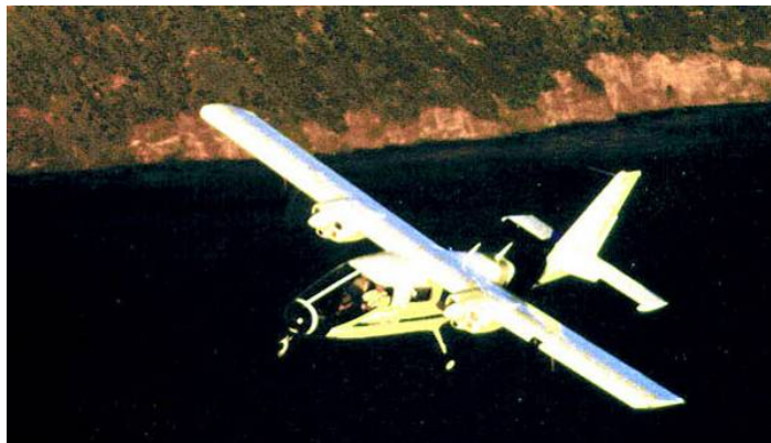
Figure 2b. The Partenavia P68 Observer fixed-wing, twin-engine aircraft used during the October-November 2008 aerial survey monitoring (note the glass nose). This plane was not available during the November 2009 surveys but is preferred to conduct surveys when it is available given the glass nose and improved sighting effectiveness from the pilot and co-pilot seats.
