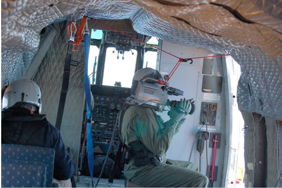
Figure 4. Extended Range Video System (ERVS). Videographer (right) is operating through an open door during flight. Note webbing restraints from ceiling attached to harnesses of all occupants. The MMO (left) was able to stand and move within the cabin to view the water through several windows on both sides of the craft, as well as through the open door.
