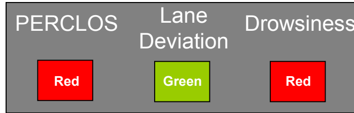
Figure 52. Expected DVI Output Display Near the End of the 10-Second “Eye Closure Only” Tasks
