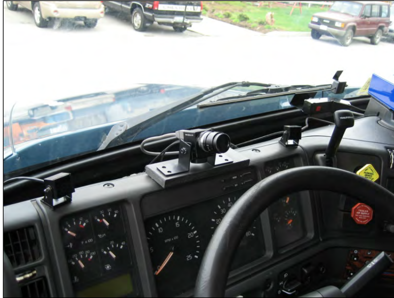
Figure 5. MV System B Infrared-Illuminator Placement
