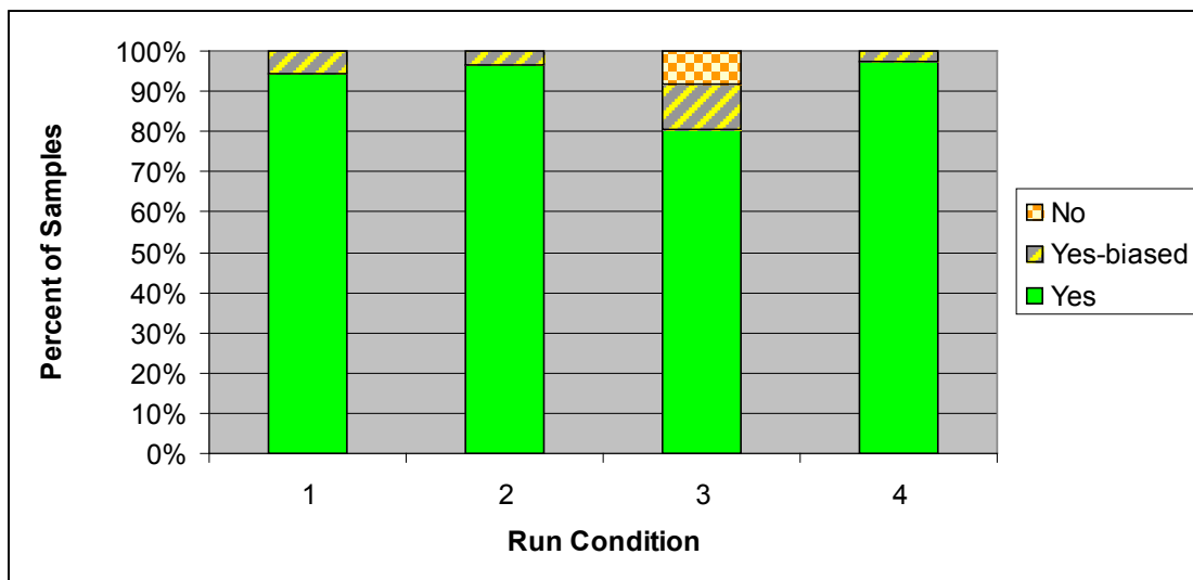
Figure 47. Overall Operational Performance of the DDMS Lane Deviation Sensor by Run Condition
