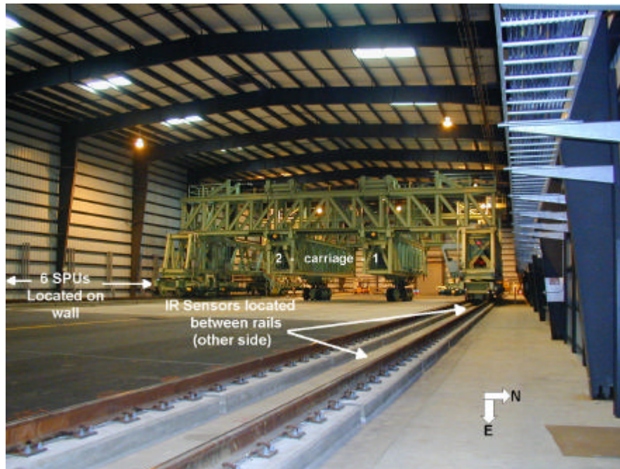
Figure 5. Test Vehicle, IR Sensor, and SPU Locations
