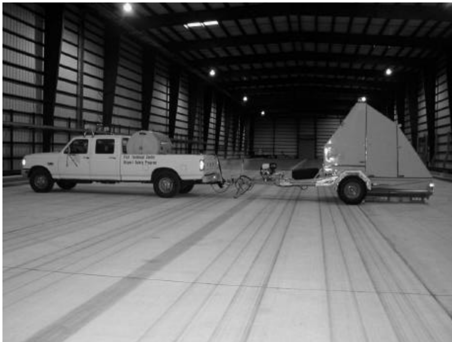
Figure 1. FAA's KUAB Model 240 HWD Equipment.
