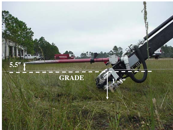
Figure 25. Below Grade Measurement
