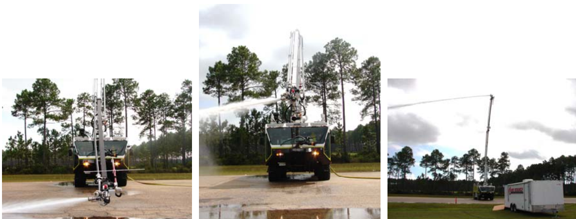
Figure 39. Oscillation Tests With Water Spray
