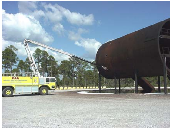
Figure 32. Penetrating the Cargo Deck
