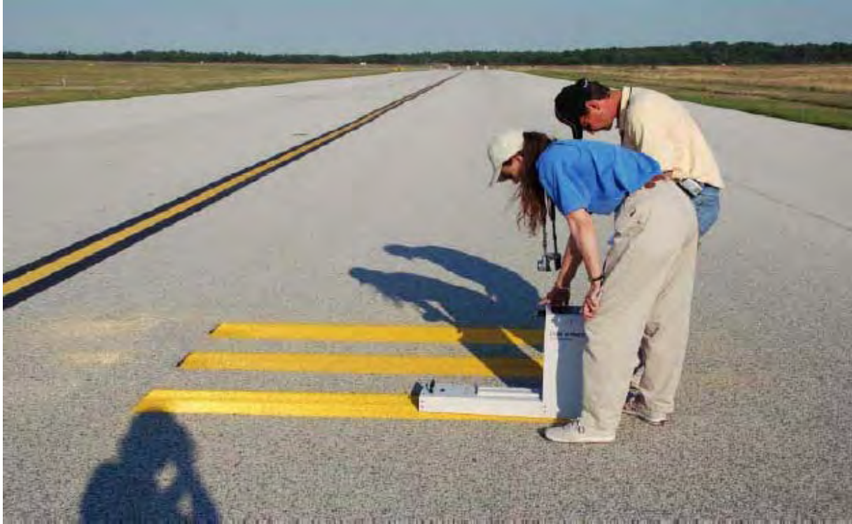
Figure 9. Applying 12" x 6' Edge Lines on Aged HMA at Test Site Three Using a Delta LTL-X Retrometer
