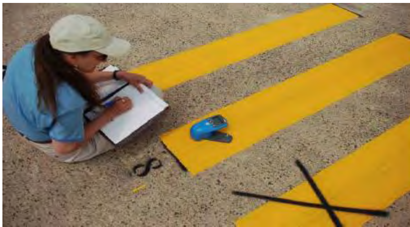
Figure 15. An FAA Airport Safety Technology R&D Sub-Team Member Taking Chromaticity Readings
