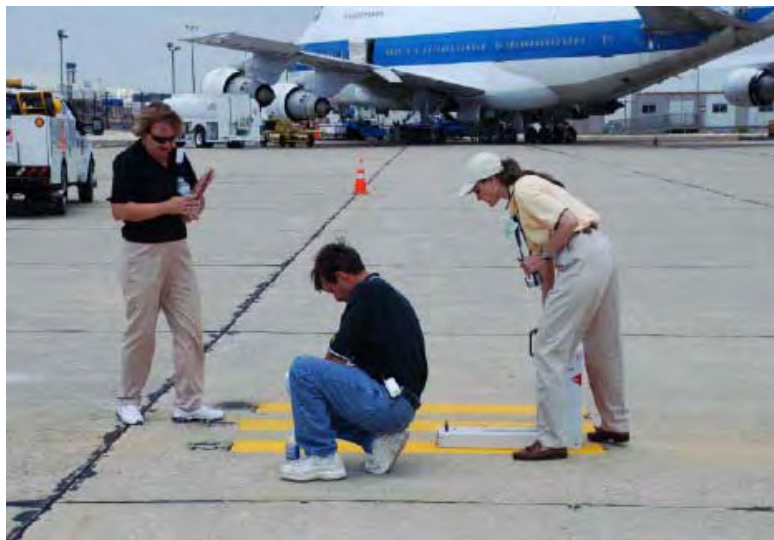
Figure 17. The FAA Airport Safety Technology R&D Sub-Team Members Taking Retro-Reflectivity Readings
