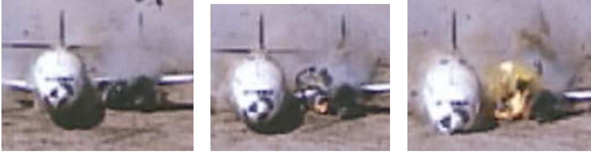
Figure 55. Video Footage of Engine Impact With the Wing Leading Edge at Tank 5 (close up)
