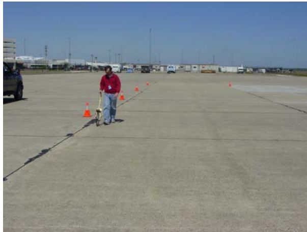
Figure 15. Setting Up Parking Cones on the Aircraft Apron for Braking Test
