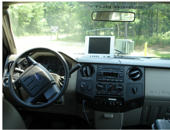
A-3. Personal Computer Installed Under the Driver's Seat With the Monitor on the Vehicle Dashboard
