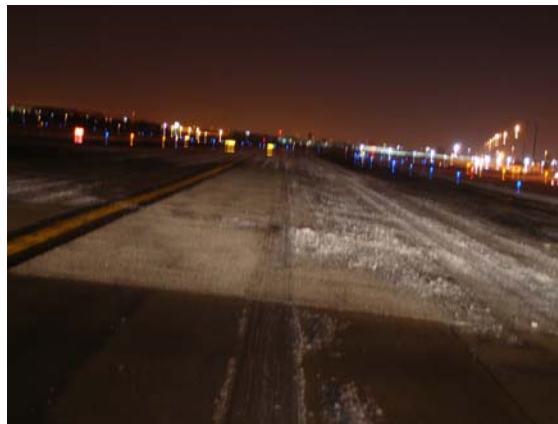
Figure 5. Ice and Slush Located on the Test Section, but not on the Adjacent Taxiway, 2/23/2005
